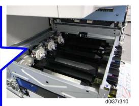
4. Take aside the ITB contact motor unit [A] (  $\mbox{\ensuremath{\beta}}\mbox{ x 2)}$
