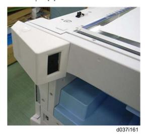
6. Peel off double sided tape on the key counter bracket, and attach the key counter to the scanner right cover.
