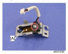
4. Heating roller thermistor [A] ( $\widehat{\mathscr{E}} \times 1$ )
