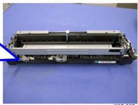
3. Thermistor end assembly [A] ( $\hat{F} \times 1$ ,  $\Box V \times 1$ )
