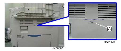
9. Close the duplex unit, and then attach the 'Push' decal [A] to the duplex unit cover.
