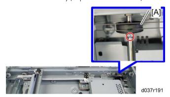
10. Rear scanner drive pulley [A] ( $\mathscr{F} \times 1$ )
