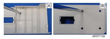
7. Make four holes in the scanner left cover with a screwdriver as shown [A].
