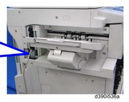
3. Attach the bracket [A] ( $\mathscr{F}$  x 2); this bracket is for the internal finisher when used with the punch unit.
