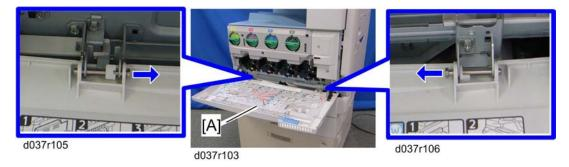
4. Front door [A] ( $\langle \overline{\langle} \rangle \times 2$ , pin x 2)
