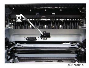
2. Clean the thermopile lens [A] with a dry cloth.
