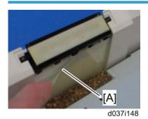
Make sure that the mylar [A] does not go under the friction pad when reinstalling the friction pad.
