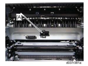
2. Clean the thermopile lens [A] with a dry cloth.
