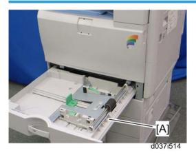
1. Pull each paper tray [A] out. Then adjust the side guides and end guide to match the paper size.
