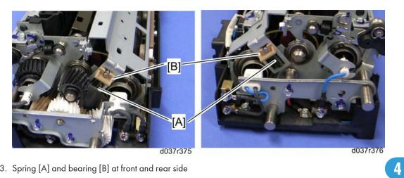
3. Spring [A] and bearing [B] at front and rear side
