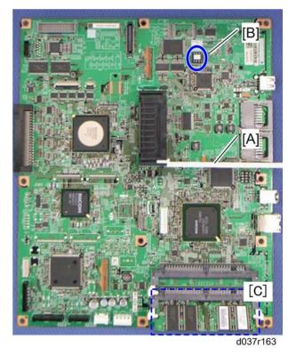
5. Remove the Interface rails [A], NVRAM [B] and RAM-DIMM [C].
