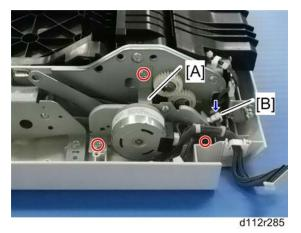
3. By-pass motor with the bracket [A] ( 🌶 x 3, 🖨 x 2, 🖽 x 1)
