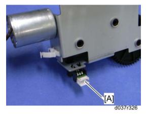
2. ITB contact sensor [A] (hooks)
