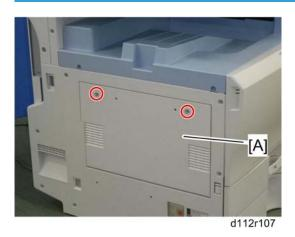
1. Open the ITB cleaning unit cover [A] ( 🌶 x 2).
