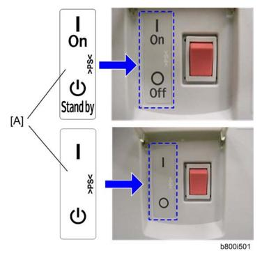
17. Attach the on/standby decal [A] to the left-hand side of the main power switch.
