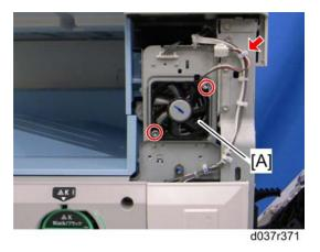
2. Fusing front fan [A] ( 🌶 x 2, 🖨 x 1, 🗂 x 1)
