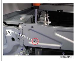
2) Check the screw position [A] as shown above.
