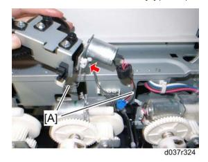
4. Disconnect two harnesses [A], and then remove the ITB contact motor unit ( $\textcircled{B} \times 1$ )
