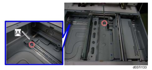
11. Move the scanner carriage to the left side as shown above by rotating the scanner motor at the rear of the machine.
