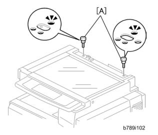
2. Insert the two stud screws [A] on the top of the machine.
