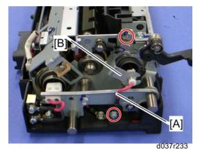
4. Remove the cable [A] from the front stay ( otin x 1).
