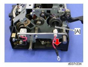
6. Pressure roller fusing lamp [A]
