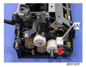
5. Heating roller fusing lamp [A]
