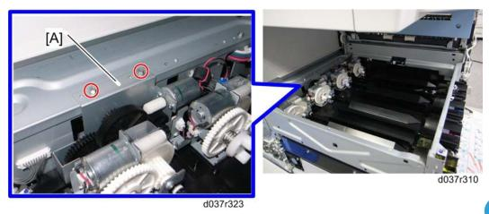
3. Take aside the ITB contact motor unit [A] (  $\checkmark$  x 2)
