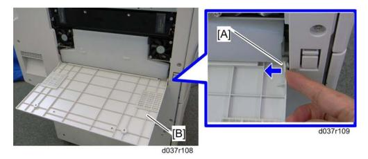
2. Release the tab [A], and then remove the ITB cleaning unit cover [B].
