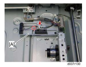
2. Original length sensor assembly [A] ( **\*** x 1, **\*** x 1, **\*** x 1 each)
