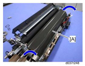
14. Fusing belt [A] with rollers
