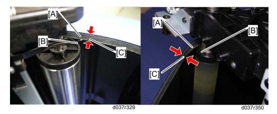
• There is a rim [A] at each edge of the transfer belt. The ends of all the rollers ([B] for example) in the transfer belt unit must be between the two rims.
