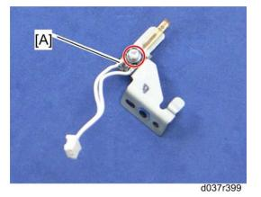
4. Pressure roller thermistor: End [A] ( 🌶 x 1)
