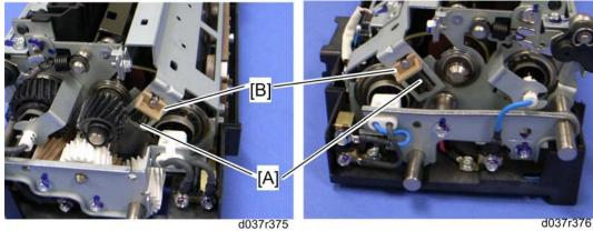
7. Spring [A] and bearing [B] at front and rear side
