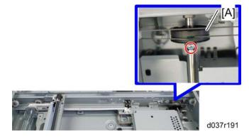
10. Rear scanner drive pulley [A] ( 🌶 x 1)
