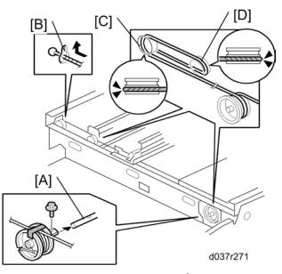
4. Install the drive pulley on the shaft [A] (  $P \times 1$ , clip x 1).
