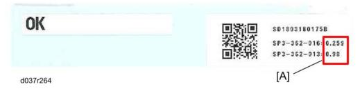
3. Input all correction coefficients [A] for the ID sensor with the SP modes referring to the barcode sheet provided with the new ID sensor unit/board.
