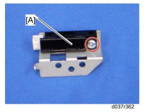
3. Fusing exit sensor [A] ( 🌶 x 1)
