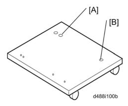
2. Install the two pins in the screw holes [A] [B].
