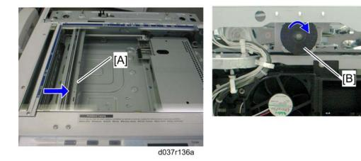
3. Move the 1st scanner carriage [A] to the right side by rotating the scanner motor [B] clockwise.
