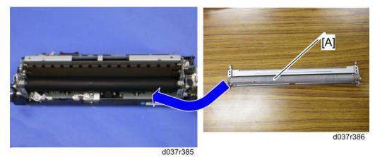
4. Install the cleaning unit [A] in the fusing unit.
