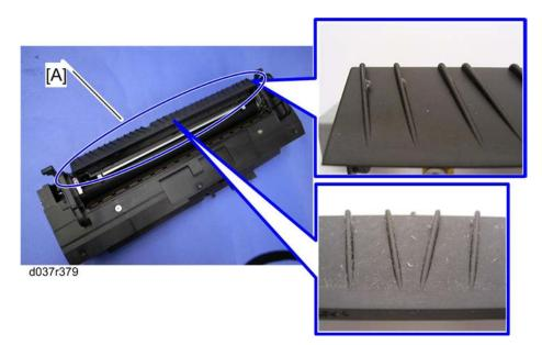
3. Clean the exit guide plate [A] with a cloth moistened with alcohol.
