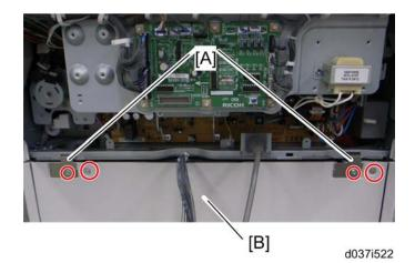
Remove the securing brackets [A] ( \* x 1 each), and then rear cover [B] of the paper feed unit ( \* x 2).
