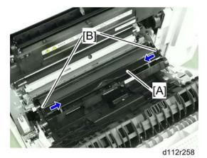
3. Remove the PTR unit [A], releasing the two locks [B].
