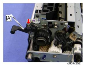
3. Pressure levers [A] at the rear side (snap ring x 1, spring x 1)
