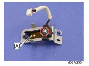
4. Heating roller thermistor [A] ( 🌶 x 1)
