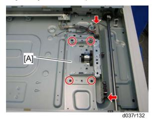
3. Sensor board unit [A] ( 🌶 x 4, ground screw x 1, 🗂 x 2)
