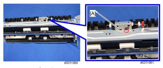
2. Sensor assembly [A] ( 🌮 x 1, 😂 x 1, 🗂 x 1)
