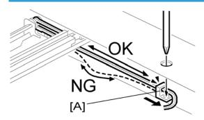
Run the cable so there is no slack. Slide the adjustor clamp [A] to adjust the cable slack.
