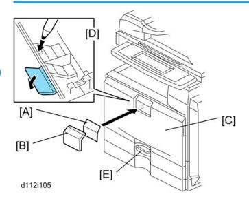
1. Attach the correct emblem [A] and the cover [B] to the front door [C] of the machine, if the emblem is not attached.
