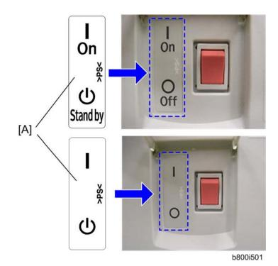
6. Attach the on/standby decal [A] to the left-hand side of the main power switch.
