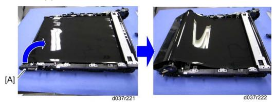
9. Pull the tension roller [A] as shown.
