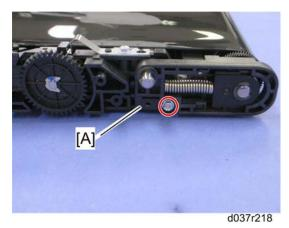
6. Rear holder bracket [A] (as seen from the rear) (  $\checkmark$  x 1: M3x10)
