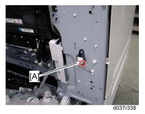
2. Temperature and humidity sensor [A] ( 🌶 x 1, 🗂 x 1, 🛱 x 1)
