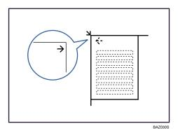
• Make sure to set the test pattern on the exposure glass, and then 2 or 3 white sheets, same size as the test pattern, above the test pattern.
