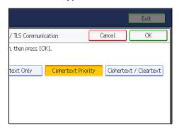
Select [Ciphertext Only], [Ciphertext Priority], or [Ciphertext / Cleartext] as the encrypted communication mode.
