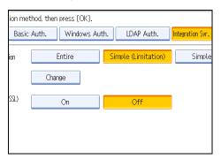
3. Specify the range in which [Simple (Limitation)] is applied to "Printer Job Authentication".
