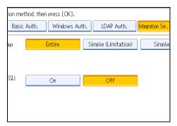
To not use secure sockets layer (SSL) for authentication, press [Off].
