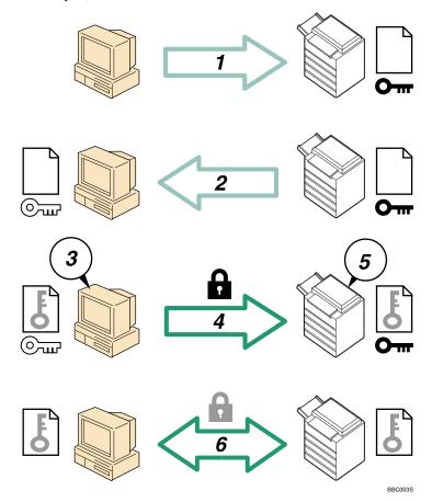
1. To access the machine from a user's computer, request the SSL device certificate and public key.
