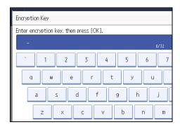
Enter the encryption key using up to 32 alphanumeric characters.
