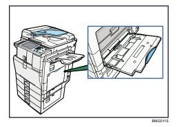
2. Gently insert paper face down into the bypass tray until the beeper sounds, and then adjust the paper guides to the paper size.
