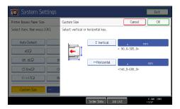
Press [Horizontal], enter the horizontal size of the paper using the number keys, and then press the [<sup>‡</sup>] key.
