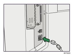
4. Connect the other end of the Ethernet interface cable to a network connection device such as a hub.
