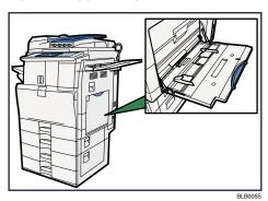
2. Insert the paper face down until you hear the beep, and then align the paper guides to the paper size.
