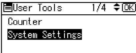
3. Press the [▼] or [▲] key to select [Interface Settings], and then press the [OK] key.
