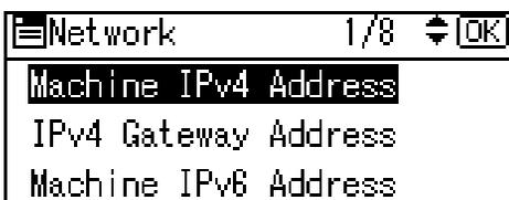
Enter the IPv4 address and subnet mask. To specify a static IPv4 address for this machine, select [Specify], and then press [IP Add.]. To specify a subnet mask, select [Specify], and then press [Subnet M].
