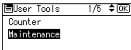
**3** Select [Clean Print-heads] using [▲] or [▼], and then press the [OK] key.
