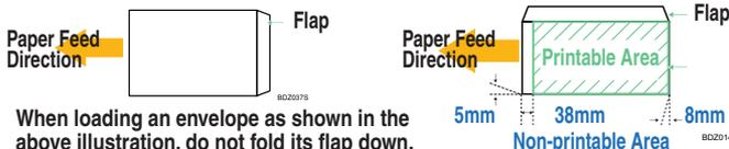
When loading an envelope as shown in the above illustration, do not fold its flap down.
