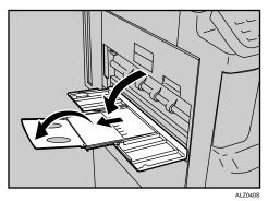
Do not open the one-sheet output tray while the machine is in operation.
