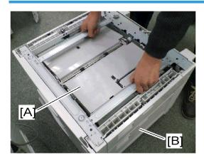
1. Set the duplex unit [A] on the paper tray unit [B] grabbing the stays at the top of the duplex unit as shown.
