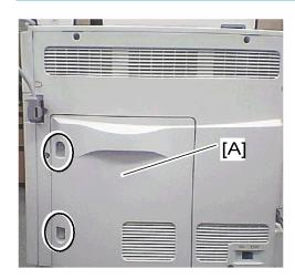
1. Rear engine unit cover [A] (locking screw x 2)
