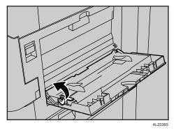
Adjust the paper guides to the paper size, and then gently insert paper face up into the bypass tray.
