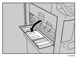
Adjust the paper guides to the paper size, and then gently insert a sheet face up into the One Sheet bypass tray.
