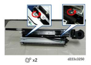
6. While holding the hopper perfectly level as you remove it to prevent toner spill, rotate the toner hopper very slightly (10° to 20°) and remove it.
