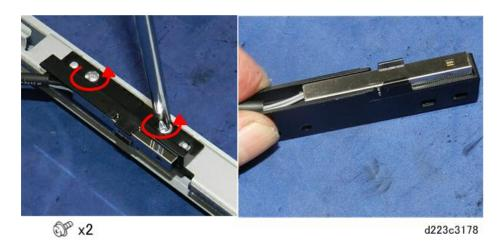
9. On the other end of the bracket, disconnect the power pack cover.
