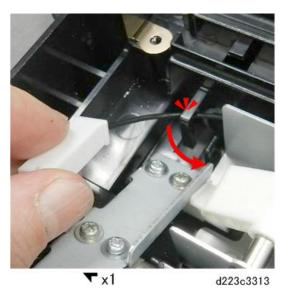
6. Remove the top screw [A] of the solenoid bracket, and then loosen the two left screws [B]. (This allows you to free the front terminal harness below the bracket at [A].)
