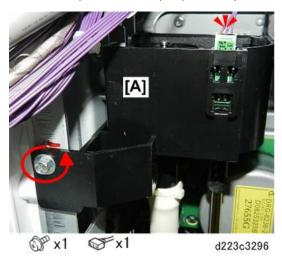
5. Pull out the stopper on the tube base [A].
