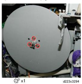
3. The used toner pump tube assembly and drive rod [A] block the removal of the motor [B].
