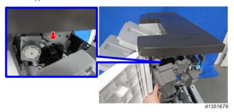
7. Remove screw [A] of the transport guide plate from the rear of the finisher.
