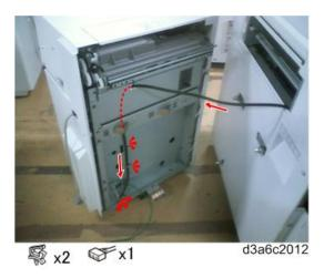
10. Connect the ground wire to the side of the main machine near the joint connector, at about a 45 degree angle as shown.
