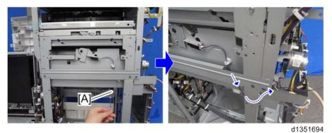
20. Route the harness of the hopper bracket to the rear of the finisher.
