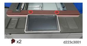
4. Bend the ends of the cover toward you slightly to disengage the tabs on the ends, and then remove the front edge cover.
