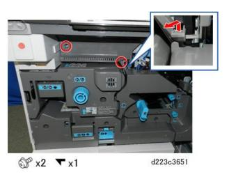
4. Disconnect the sensor harness and sensor bracket.
