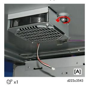
9. From the left side of the machine, disconnect the fan bracket [A], and then remove the bracket with fan attached from the machine [B].
