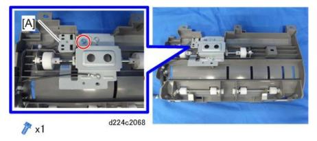
3. Separation Sensor [A] and Skew Correction Sensor [B].
