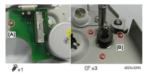
24. Separate the motor and base motor bracket.
