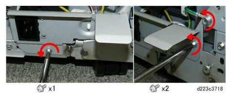
6. Pull the plate away from the corner of the machine. Do not remove it.
