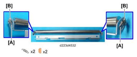
3. Separate the roller and bracket.
