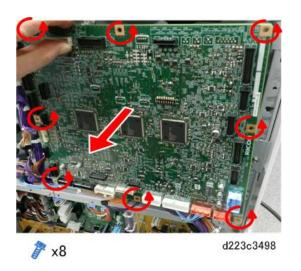
10. Lay the board on a flat clean surface.
