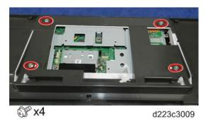
10. Lift the operation panel cover up and remove it.
