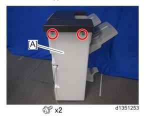
3. Remove the rear lower cover [A] of the finisher.
