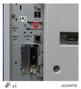
6. Insert the flat connector of the accessory USB cable [A] into the **USB-A** connector on the interface board.
