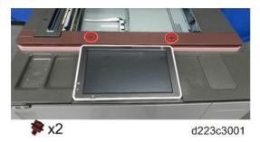
3. Bend the ends of the cover toward you slightly to disengage the tabs on the ends, and then remove the cover.
