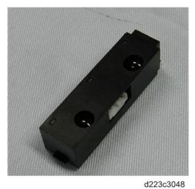
6. Press the back right sensor [A] to release it, and then disconnect it.
