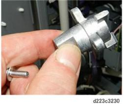
6. Remove the small gear. (This gear is black in the D223/D224, and white in the D225.)
