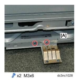
13. Set the tab [1] and boss [2] of the ground plate extension on the bottom edge, and then fasten it with the screws.
