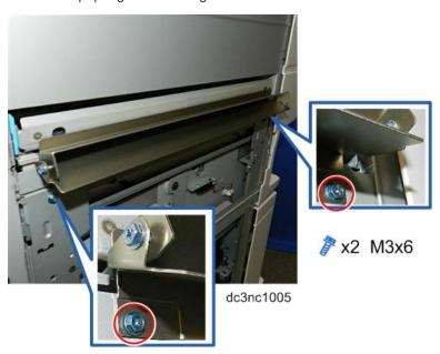
2. If the finisher is the Booklet Finisher SR4130, remove the upper right plate [A]. (The Finisher SR4120 does not have this plate.)
