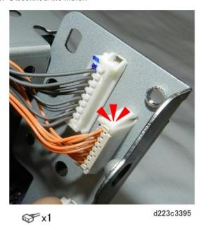
5. Disconnect the motor cover plate at the front [A] and at the rear [B].
