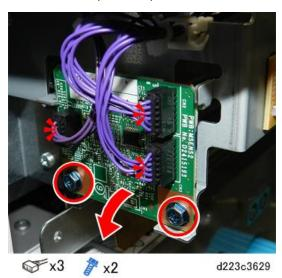
9. Unfasten the detection device bracket, and then pull it out partially.
