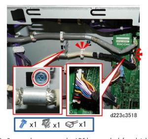
9. Remove the screws on the ADF base on the left and right.
