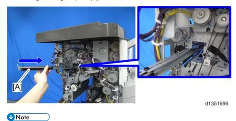
• Hook [A] and [B] of the registration guide plate onto the slotted holes of the finisher.
