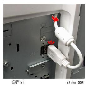
16. Pass the cable over the left, rear corner [A], and then clamp it to the left side of the frame [B].
