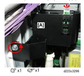
11. Pull out the stopper on the tube base [A].
