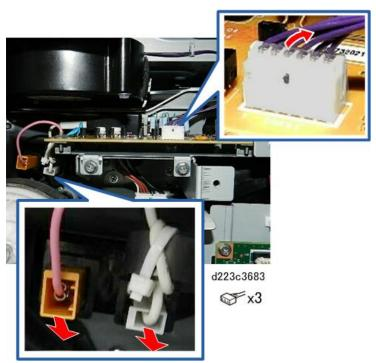
9. Disconnect the power pack bracket, and then remove it with the power pack attached.
