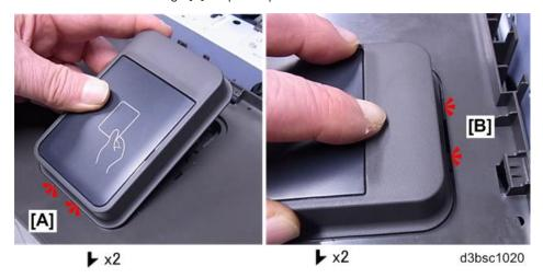
27. This completes the installation. Re-attach the operation panel.
