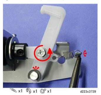
5. Disconnect and then remove the mounting plate.
