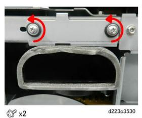
4. Pull the duct and fan out slightly, and then disconnect the fan.
