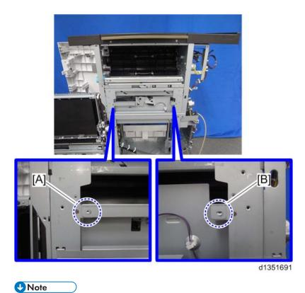
• Make sure the hooks [A] and [B] of the hopper bracket are also hooked onto the finisher.
