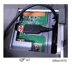
18. Set the cable in the notch of the frame [A].
