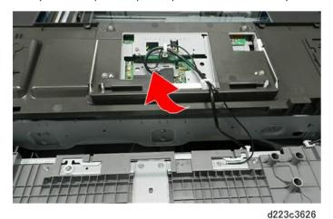
7. This detection device [1] and PCB [2] comprise the sensor.
