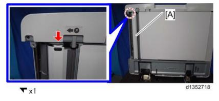
3. Note that the tabs [A] on the ends of the non-contact scanning guide plate (just removed) are black, and the tabs [B] (replacement) of the contact-type are white.
