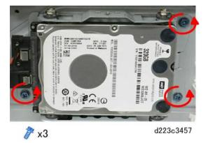
6. Unhook the HDD bracket from the machine frame.
