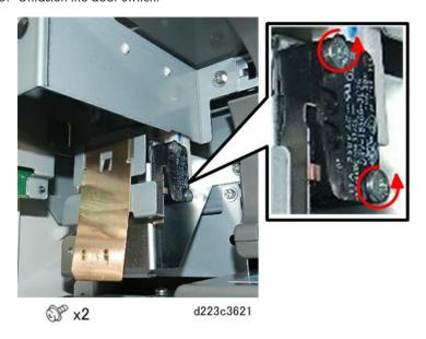
4. Disconnect the door switch bayonet connector.
