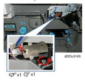
4. Without touching the wire mesh on top of the unit, pull the charge corona unit out of the machine.
