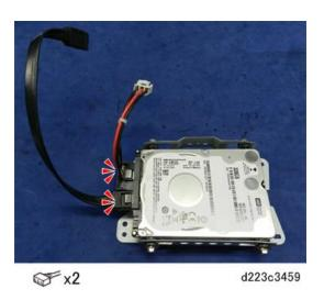
8. Remove the screws from the bracket front [A] and rear [B].
