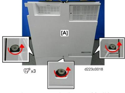
10. Disconnect the rear upper cover at the right rear corner [A] and left rear corner [B].
