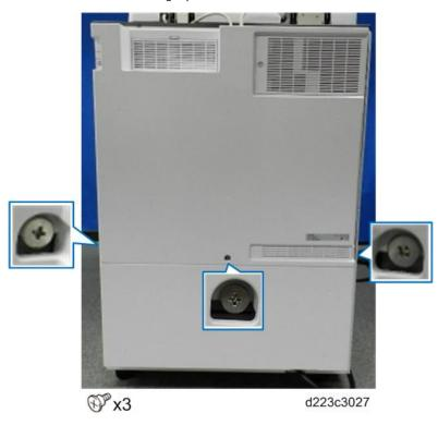
1. Disconnect the cover at the right upper corner [A] and left upper corner [B]. Remove these screws.
