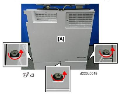
2. Disconnect the rear upper cover at the right rear corner [A] and left rear corner [B].
