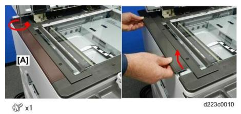
5. At the back of the scanner unit, remove the rear edge plate (no screws).
