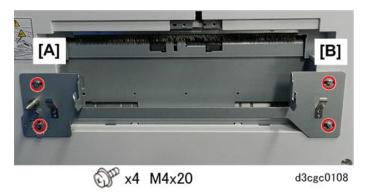
2. With the joint bracket [A] floating freely on the loose screws, move the bracket to position screw [B] so it is centered exactly below the long line on the scale, and then tighten the four screws.
