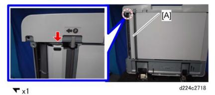
3. Original registration sensor [A] along with the bracket.
