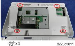
3. There are small tabs on the cover at [1] and [2]. Separate the cover and remove it,
