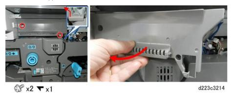
3. With the cover removed you can see the duct of the toner bottle fan.
