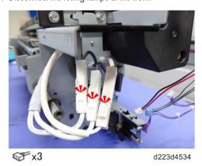
10. Remove the fusing lamp holder from the front.
