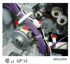
14. On the right side of the machine, disconnect the frame of the bypass unit.
