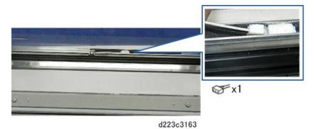
8. Roll the PTL bracket out from under the edge of the frame.
