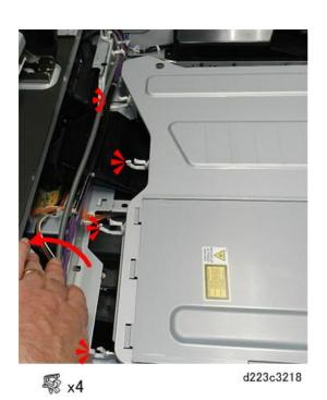
10. Pull the cover [A] away from the front edge of the machine [B] . (You do not need to remove.)
