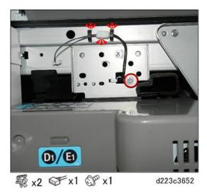
5. Remove the sensor bracket with sensor attached.
