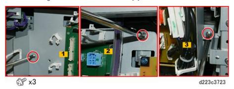
13. Continue to disconnect the mounting plate near fan [1] and then fan [2].
