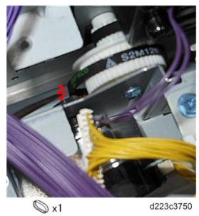
7. Disconnect the motor and remove it.
