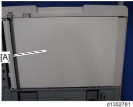
2. Put the white cover [A] in the correct position on the exposure glass, aligning it with the glass cover [B] and the rear scale [C].
