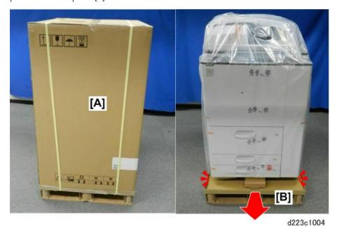
3. Remove visible orange tape and cardboard strips from the front [A] and right side [B] of the main machine.
