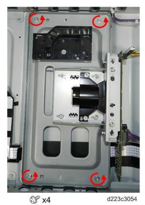
• Never loosen or attempt to remove a paint-locked screw on the lens block.
