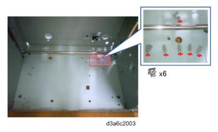
20. Set the LCIT heater, and then pass the heater harness under the rear side of the shaft.
