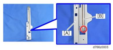
4. Remove the paper output cover [A] ( x 2).
