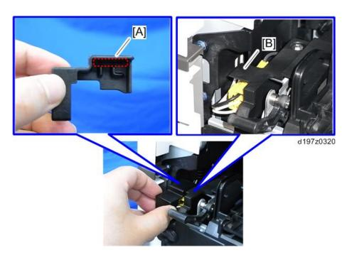
• The connector cover must be attached **before** screwing in the fusing unit.
