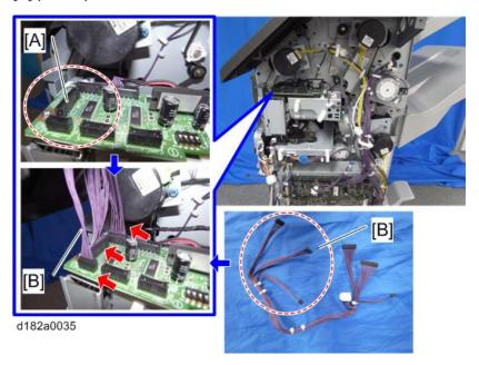
25. Connect the harness [B] provided as an accessory, to the main board [A] of the finisher (Fx3).
