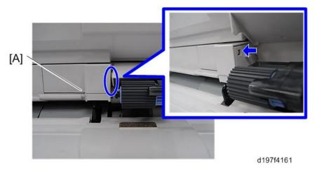
3. Bypass paper end sensor unit [A] (@x1, @x1)
