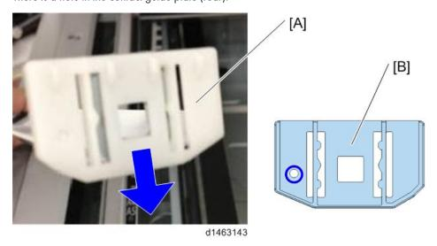
5. Attach the document reader guide plate. Be careful not to scratch the sheet [A].
