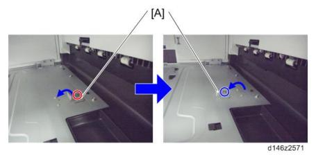
4. Replace the lock holder of the bottom plate with the lock holder [A] provided (\$\mathbb{O}^\* \times 1).
