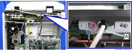
33. Remove the SIO board [A] if the DF is installed (@x4, @x6, flat cable x1).
