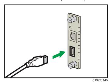
5. Insert the other side of the USB cable into the USB port B on the main machine.
