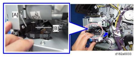
23. Secure the punch drive motor [A] ( x2).
