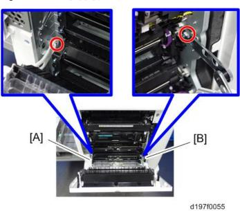
7. Slide to the left and remove right cover [A] (\$\mathbb{B} \times 1).
