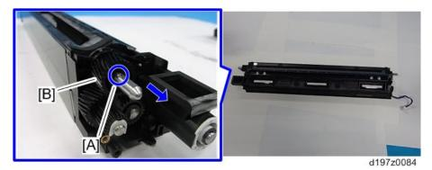
3. Gears [A] [B] (\$\text{\$\partial} \times 1, E-ring x1)
