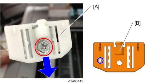
4. Replace the contactless guide plate (rear) [A] with the contact guide plate (rear) [B].
