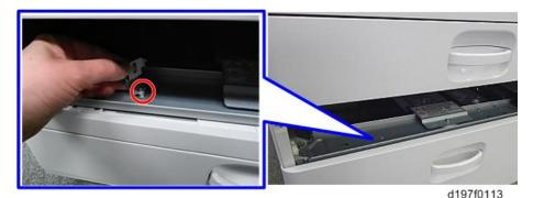
6. Attach the securing brackets [A] to two positions on the left and right at the rear of the machine (screws: 1 each).
