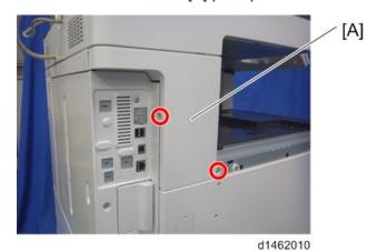
10. Remove the inverter tray [A] and tray support rod cover [B] (0°×1).
