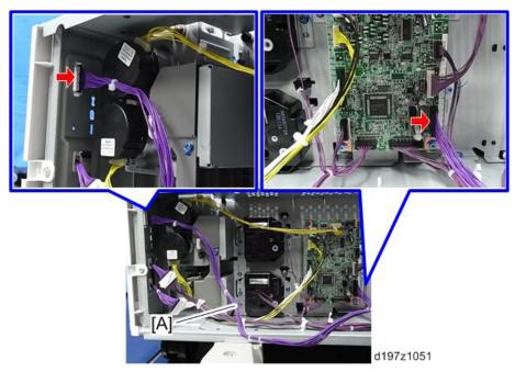
Clamp the harness (PB3170/ PB3230: <sup>®</sup>×9, PB3210/ PB3220: <sup>®</sup>×5).
