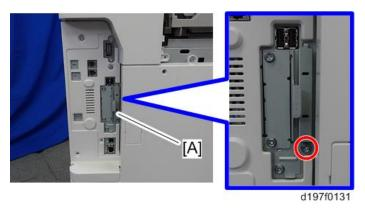
4. Insert the SD card into SD slot 2 [A].
