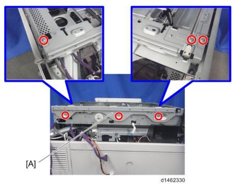
7. Move the 1st scanner carriage to the set position of the scanner fixing pin.
