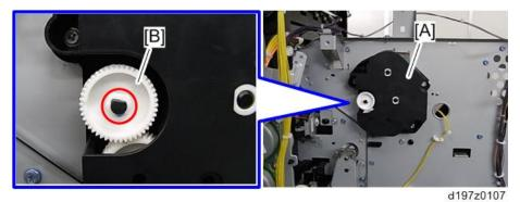
5. Screws and tab on the gearbox [A] (@x3, tabx1)
