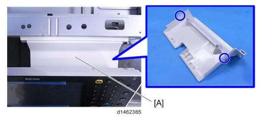
6. Remove the standard operation panel [A] (\$\mathfrak{O}^{\times} \times 5, \$\mathfrak{S}^{\times} \times 2\$).
