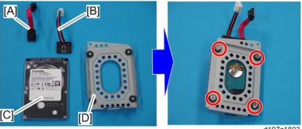
3. Connect the cables of the HDD to the controller board [A], and then hang the HDD [B] on the hook of the controller box (\$\sigma x2\$).
