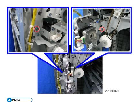
• Insert the front pins of the registration mobile unit into the holes of the frame.
