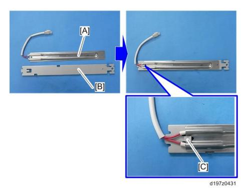
8. Attach the thermostat [A] to the Anti-condensation heater (PCU) [B] ( $\mathfrak{G}^*x1$ ).
