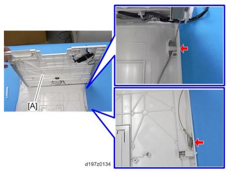
6. Bypass width sensor [A] (❤ ×1, ▼ x2)
