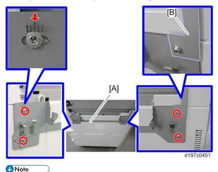
• When adjusting registration, change the screw hole of the adjusting bracket [A] from the upper position [B] to the rear (left) position [C] so that the adjusting bracket can be adjusted horizontally.
