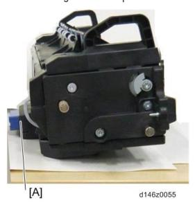
2. Move the shield drive gear with your hands to put the upper surface of the feeler [A] in a horizontal position.
