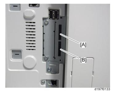
[A]: SD card slot 1 (option slot)[B]: SD card slot 2 (service slot)
