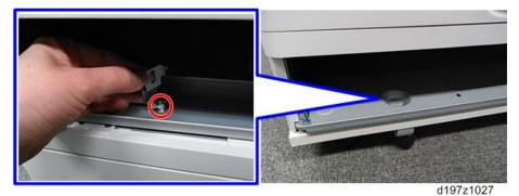
5. Install the securing bracket [A] at the rear of the PB3150 ( $\mathfrak{S}^{*}$ ×2)
