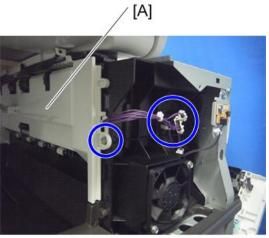
14. Open the harness cover [A], then remove the harness [B].
