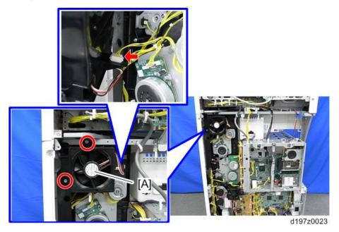
3. Fusing exhaust heat fan [A] ( ×4)
