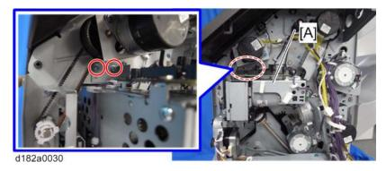
22. Insert the punch drive motor from the rear of the finisher.
