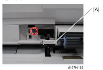
4. Bypass paper end sensor [A] (hooks)
