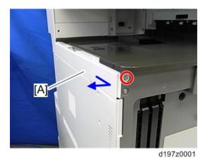
4. Remove the controller cover [A] (\$\mathscr{O}^\* \times 4\$).
