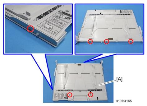
3. Release the hooks around the bypass tray [A]
