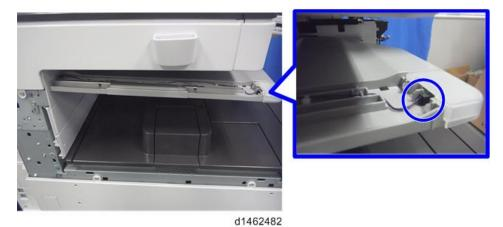
19. Insert the tray support bar firmly in the 1 bin tray, and attach the harness cover [A].
