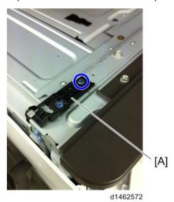
5. Fasten the bottom plate with screws (\$\mathbb{O}^2 \times 3).
