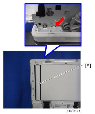
Replace the contactless guide plate (front) [A] with the contact guide plate (front) [B] ( \( \sigma \) \)
