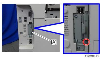
2. Put the SD card containing the firmware to install in SD card slot 2 [A].
