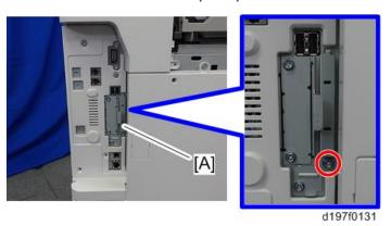
3. Insert the SD card (DataOverwriteSecurity Unit) in SD slot 1 (upper) [A] with its label face towards the front of the machine. Then push it slowly into SD slot 1 (upper) until you hear a click.
