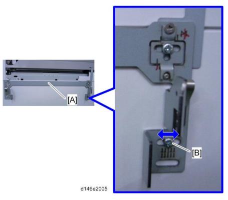
1. Eject a sheet of A4(LEF) or A3 A4(LEF) paper to the proof tray and check for how many divisions of the scale the edge of the paper has shifted from the center.
