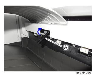
21. Slide the finisher [A] along the rail of the bottom plate from the left side of the machine, and then attach it ( \*1).
