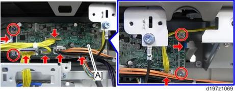
34. Connect the heater cable [B] which is shown in step 29 to another harness [A] which is shown in step 19.
