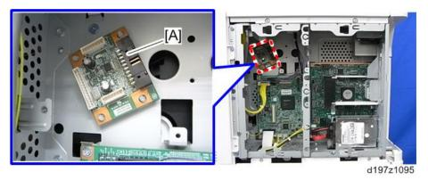
4. Connect the supplied harness (13 pins) to CN3 [A] on the optional counter interface board and CN132 [A] on the BCU.
