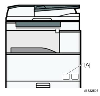
18. Connect the Ethernet cable to the Ethernet I/F [A].
