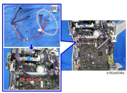
26. Connect the harness [B], provided as an accessory, to the harness of the registration sensor unit [A] ( x1).
