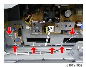
14. Connect the harness [A] to CN121 of the BCU and CN930 of the heater board.
