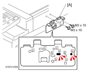
6. Attach the lower tray [A] to the tray bracket ( $@x2: M3 \times 8$ ).
