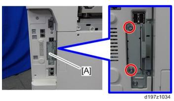
2. Install the board of the file format converter in the I/F slot [A] ( \$\mathbb{O}^{\mathbb{C}} x2 ).
