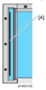
2. Wipe the exposure glass with alcohols so that no glue remains from the double-sided tape.
