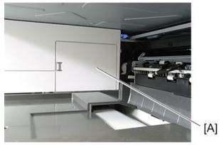
17. Remove the paper exit lower cover [A] (\$\mathscr{O}^{\pi} \times 2).
