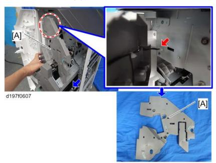
9. Open the upper cover [A] and remove the arm of the guide plate [B] from the finisher upper cover (\$\tilde{\mathbb{R}} x 1\$).
