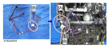
27. Remove the harness [A] from the clamp [B], and connect it to the main board of the punch unit [C] (Fx1).
