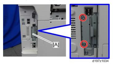
2. Install the IEEE 1284 Interface Board in the I/F slot [A] (@x2).
