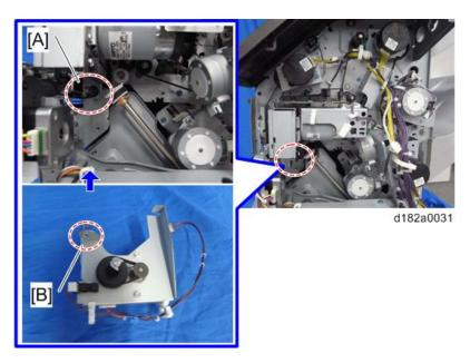
• Make sure that the rack of the punch unit [A] and the pinion of the bracket [B] are correctly engaged with each other.
