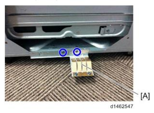
10. Attach the joint bracket [A] to the machine (\$\mathbb{O}^\* \times 4\$).
