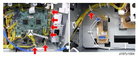
16. Connect the heater harness [A] to CN921 of the heater board, and then attach the plug-in of the heater harness to the rear frame of the main unit.
