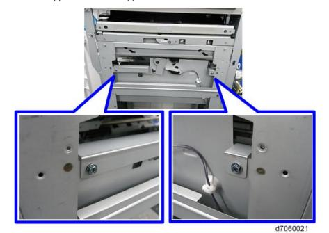
8. Connect the harness of the hopper sensor (\$\sim\$x1).
