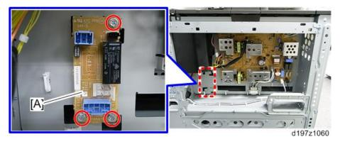
14. Connect the harness [A] to CN904 of the PSU and CN920 of the heater board.
