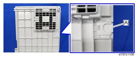
13. Pass the harness from the key counter through the cut off part [A] of the right rear cover.
