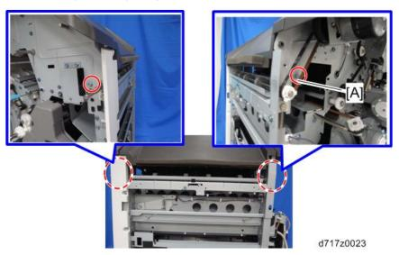
17. Insert the registration sensor unit [A] from the rear.
