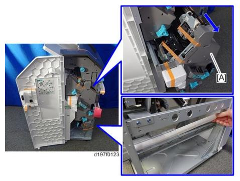
6. Wipe the surface of the top cover with alcohol, and then attach the cushion [A] (supplied with the finisher adapter) to the top cover.
