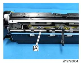
3. Paper exit sensor with bracket [A] (@\*x1, \$\simex2)
