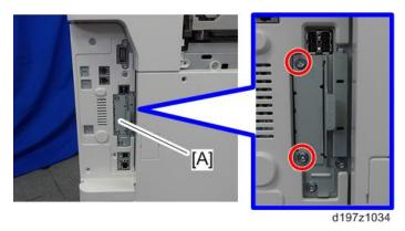
2. Install the IEEE 802.11 interface board in the I/F slot [A] (@x2).
