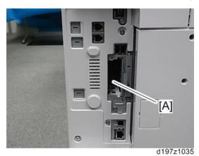
4. Insert the USB cable into the USB port on this option.
