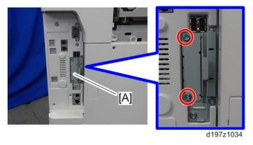
3. Install the interface board in the interface slot [A] ( $\mathfrak{S}^{r}x$  2).
