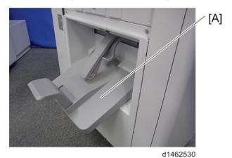
9. Attach the relay guide plate [A] supplied with the finisher adapter to the finisher (5 x 2 (M3 x 6)).
