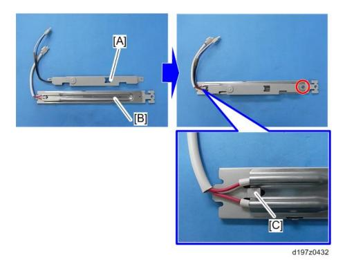
9. Put back the anti-condensation heater (PCU) [A], and then pass the heater harnesses out through the opening [B] at the inner rear side of the main unit.
