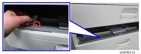
6. Attach the securing brackets [A] to two positions on the left and right at the rear of the machine (screws: 1 each).
