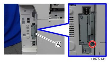
3. Insert the SD card in the service slot [A].
