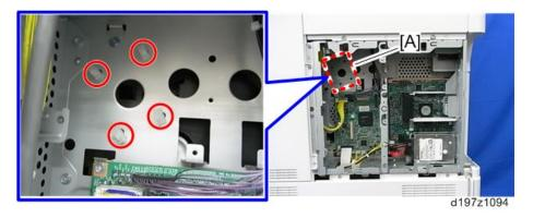
3. Install the optional counter interface board [A] on the four stud stays.
