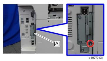
3. Insert the IPDS SD card in SD card slot 1 [A] or 2 [B].
