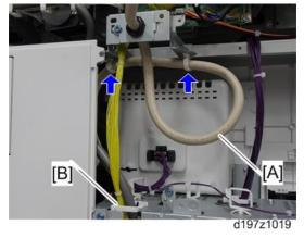
13. Attach the CIS cable clamp [A] to the bracket in the controller box (\$\mathbb{O}^{\text{x}} \text{1}).
