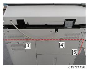
${\bf 9.}\;$  Clamp the USB cable and connect it to the USB connector.
