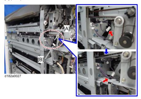
20. Insert the punch unit [A] from the rear.
