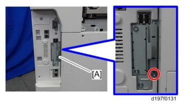
3. Insert the browser unit SD card in SD card slot 1 [A] or slot 2 [B].
