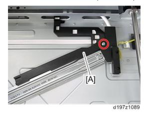
32. Remove the DF harness with the bracket [A] if the DF is installed ( $\Im x1$ ).
