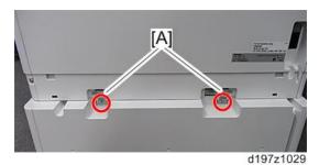
8. Attach the rear lower gap cover [A] (\(\neg x 2\))
