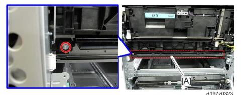
3. Release the tab on the paper dust collection unit [A] ( $\nabla \times 1$ ).
