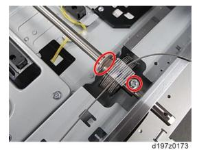
8. Attach the scanner drive gear [A], and then tighten the scanner motor bracket (5°×3, spring ×1, belt ×1).
