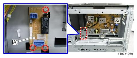
12. Connect the harness [A] to CN904 of the PSU and CN920 of the heater board.
