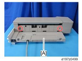
2. Release the clamp and disconnect the harness of the paper output full sensor 1 [A].
