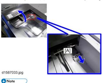
• After the stamp installation, be sure to slide the holder in correctly. If not, jam detection (J001) will occur.
