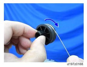
4. Coil up the ball-shaped end of the wire clockwise (when looking at the boss of the pulley)
