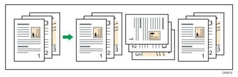
To use the Rotate Sort function, two paper trays loaded with paper of the same size and type, but in different orientation ( $\square\square$ ), are required. For details, see "Tray Paper Settings", Connecting the Machine/ System Settings.
