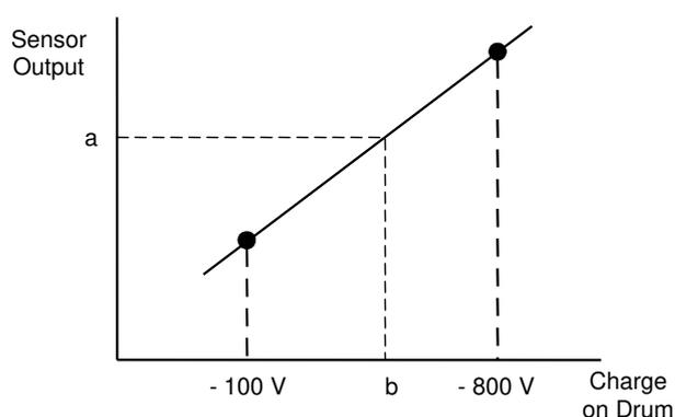
*Service manual, section 6.8.11, Drum Potential Sensor Calibration*
