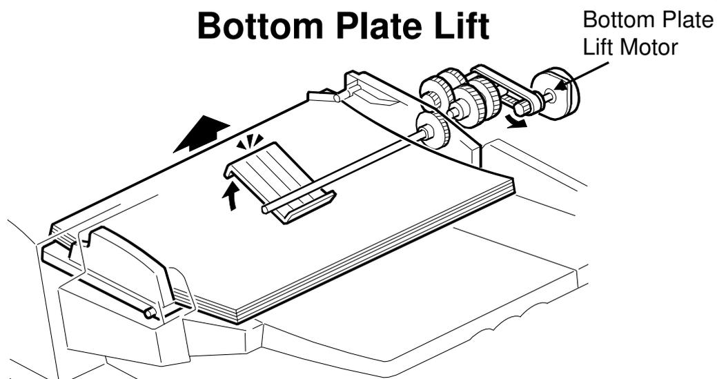
■ **The bottom plate lift motor lifts the bottom plate at the following times:**
