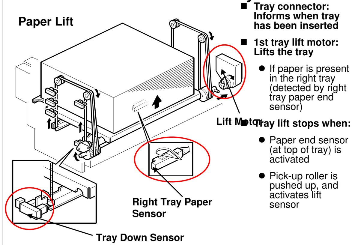
*Service manual, section 6.11.8, Paper Lift/Remaining Paper Detection*
