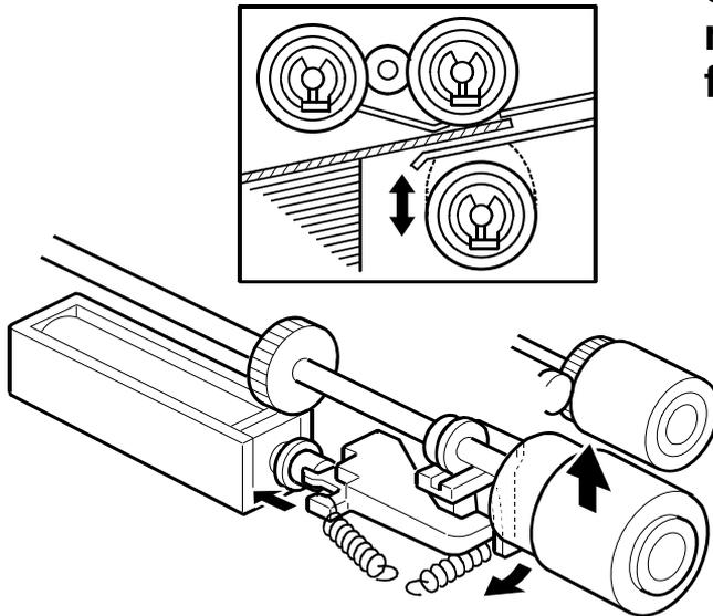
*Service manual, section 6.11.3, Separation Roller Release*
