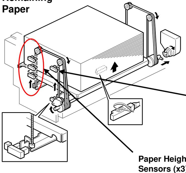
■ Paper height and near-end sensors: Detect amount of paper remaining
