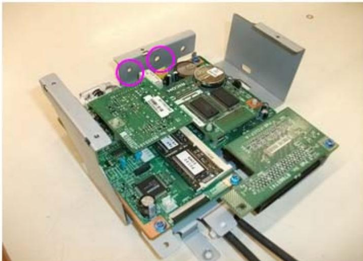
4. Attach the MBU holding bracket (screw x 1).
