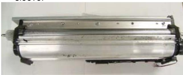
3. Clean the development roller sleeve by sliding the brush shown in the photo firmly along the entire length of the sleeve.
