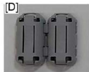
5.10 Attach the ferrite core [A] to the cables [B] on the speaker unit, and then clamp the cables.
