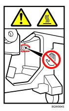
Do not touch the parts a label indicates. The inside of the Multi-Folding Unit could be very hot. Caution should be taken when removing misfed paper.
