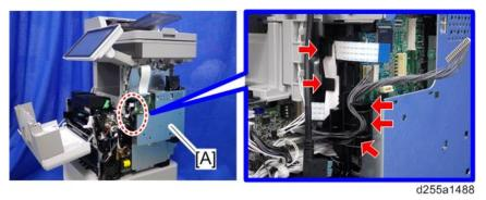
• When reattaching the bracket [A] of the controller box [B], do not interpose the harness and the flat cable between the bracket and the controller box.
