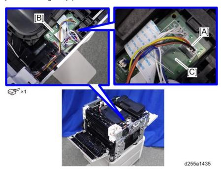
4. Release the harness [A], disconnected in the previous step, from the harness guides.
