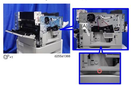
3. Release the hook by opening the right side of the left lower cover as shown below, and then remove the left lower cover [A]. (hook×3)
