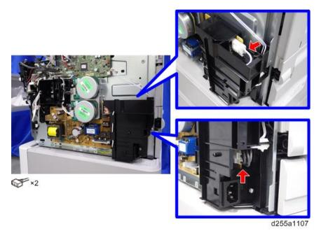
5. Remove the PSU [A] and bracket [B] from the mainframe. (hook×3)
