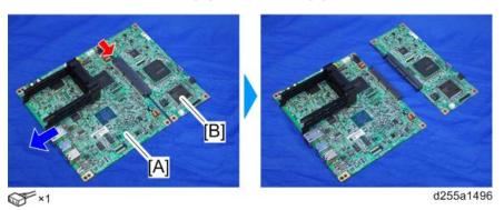
9. Remove the two guide rails [A] from the controller board [B]. (hook×2)
