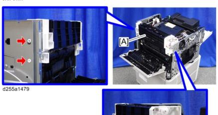
• When removing the paper exit unit [A], disconnect the connector [B] from the paper exit unit.
