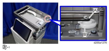
4. Remove the plate [A] and carriage belt [B].
