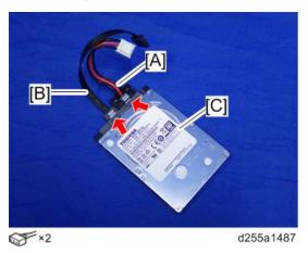
25. Install the enhanced security HDD [A] on the HDD bracket [B] with the stepped screws.
