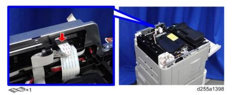
4. Remove the flat cable with the bracket [A] by sliding it to the rear while pushing the hook [B].
