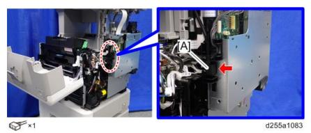
4. Disconnect the two flat cables and two connectors.
