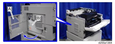
4. Release the hook by lifting the left upper cover [A] upward.
