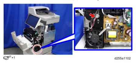
3. Release the hook [A] by lifting the fan bracket [B]. (hook×1)
