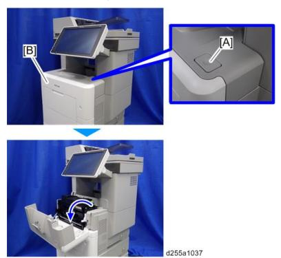
7. Release the hook [A] of the right upper cover [B] by opening the cover in the direction of the arrow.
