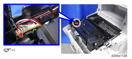
Release the hook [A] by pressing the lock lever, and then remove the development unit
