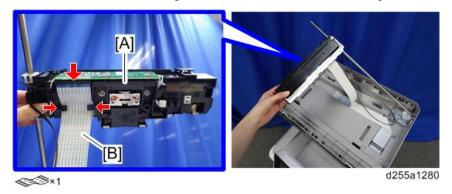
7. Remove the shaft [A] from the scanner carriage [B].
