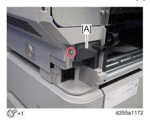
7. Release the hook, and then remove the connector cover [A].
