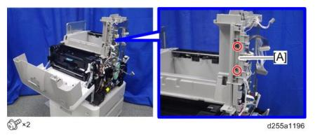
13. Remove the two screws from the right side cover [A].
