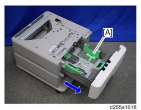
8. Install the joint bracket C [A] on the front side to secure the upper paper feed unit and lower paper feed unit with the tapping bind screw (3×8).
