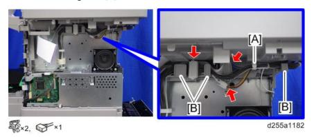
5. Remove the ground screw [A].
