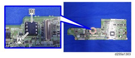
• Install a NVRAM [A] so that the indentation [B] on the NVRAM corresponds with the mark on the IOB. Incorrect installation of the NVRAM will damage both the IOB and NVRAM.
