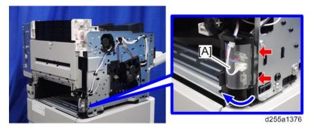
4. Disconnect the two connectors, and then release them from the harness guide [A].
