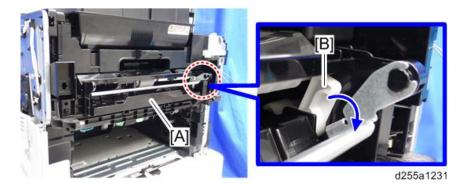
3. Slide the shaft [A] of the bypass tray paper feed roller [B] to the right while releasing the hook.
