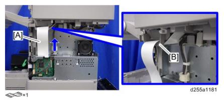
4. Open the clamp [A] and disconnect the three connectors. Then release the connectors from the harness guides [B].
