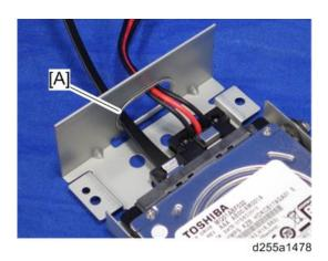
26. Install the HDD with the bracket [A] on the controller box [B] with the tapping screws. (hook×2)
