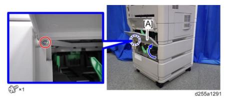
7. Remove the paper feed tray [A] of the main machine by pulling it out.
