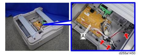
6. Disconnect the five connectors from the main board [A].
