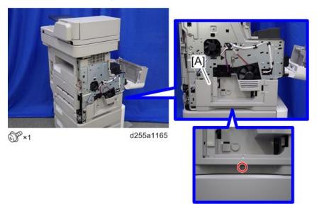
3. Release the hook by opening the right side of the left lower cover as shown below, and then remove the left lower cover [A]. (hook×3)
