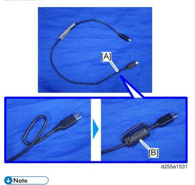
• Attach the ferrite core at a distance of 4.0 cm (1.6 inch) [A] from the end of USB cable.
