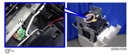
3. Turn over the fusing thermistor connection PCB [A], and then disconnect the flat cable and connectors.
