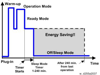
The area shaded grey in this diagram represents the amount of energy that is saved when the timers are at the default settings. If the timers are changed, then the energy saved will be different. For example, if the timers are all set to 240 min., the grey area will disappear, and no energy is saved before 240 min. expires.
