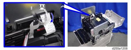
4. Remove the flat cable with the bracket [A] by sliding it to the rear while pushing the hook [B].
