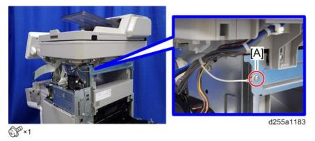
6. Remove the two screws from the rear side of the scanner unit [A].
