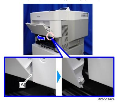
5. Remove the right connecting arm [A] and left connecting arm [B] of the bypass tray [C].
