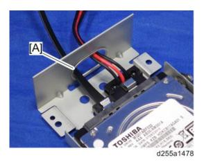
24. Install the HDD [A] on the controller box [B] with the tapping screws. (hook×2)
