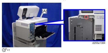
4. Lift the upper cover [A] by releasing the two hooks, and then put it on the mainframe so that you can access the bracket [B] on the right side of the machine.
