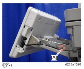
21. Install the FG clamp [A] to the operation panel arm.
