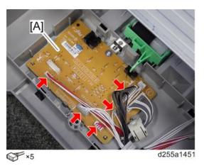
Turn over the optional paper feed unit again, and then remove the upper cover [A]. (hook×1)
