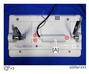
10. Remove the rear right cover [A] and rear left cover [B].
