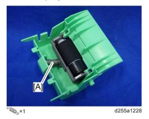
4. Remove the separation roller [A] by rotating it as shown below.
