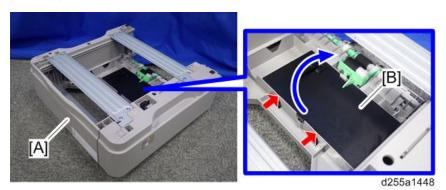
5. Release the harness of the main board [A] from the harness guides.
