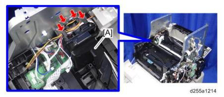
6. Remove the laser fan unit [A]. (hook×1)
