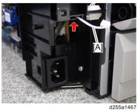
8. Remove the ground screw [A] and disconnect the two connectors.
