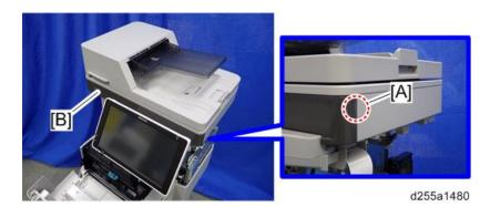
10. Release the two hooks of the scanner front cover [A].
