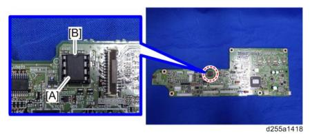
Install a NVRAM [A] so that the indentation [B] on the NVRAM corresponds with the mark on the IOB. Incorrect installation of the NVRAM will damage both the IOB and NVRAM.
