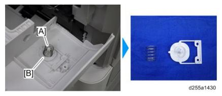
12. Remove the front cover [A] by releasing the left hinge [B].
