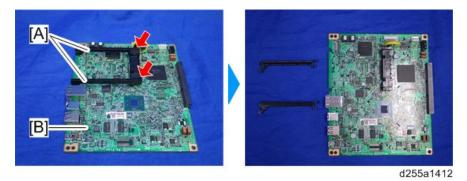
Remove the two NVRAMs [A] from the old controller board and install them on the new controller board.
