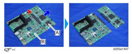
3. Remove the NVRAM [A] from the old BiCU and attach it to the new BiCU.
