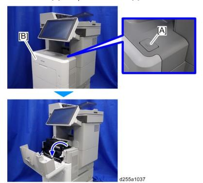
3. Release the hook [A] of the right upper cover [B] by opening the cover in the direction of the arrow.
