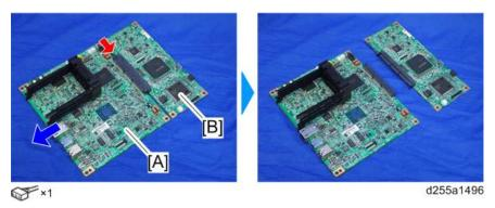
7. Remove the two guide rails [A] from the controller board [B]. (hook×2)
