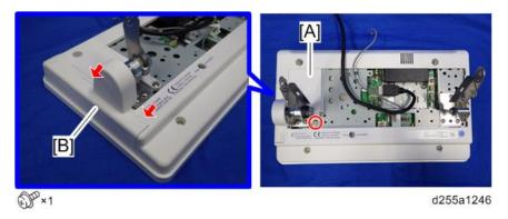
13. Remove the right hinge [A] and left hinge [B].
