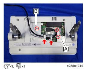
11. Remove the right hinge cover [A] and left hinge cover (lower) [B].
