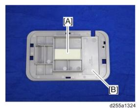
23. Peel off the mount from the hook and loop fastener, and then attach the NFC card reader [A] to the base cover [B] at the position shown below.
