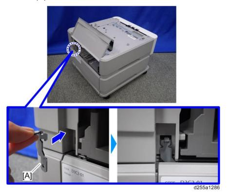
6. Open the rear cover [A] of the lower paper feed unit, and then secure the joint bracket installed in the previous step with the screw (M3×6).
