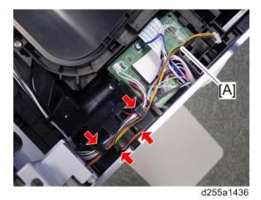
5. Remove the three screws from the left side of the machine.
