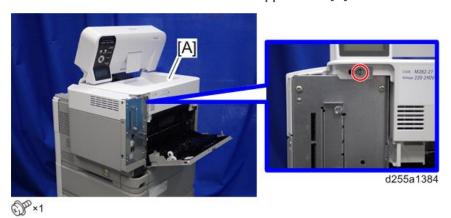
5. Lift the upper cover [A] by releasing the two hooks, and then put it on the mainframe so that you can access the bracket [B] on the right side of the machine.
