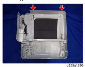
8. Remove the paper feed tray [A] by pulling it out.
