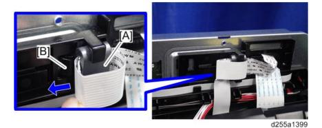
5. Pull the red harness [A] out through the apertures, and then release it from the harness guides.
