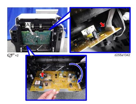
• When installing the power pack, insert the actuator [A] through the hole [B] of the power pack [C].
