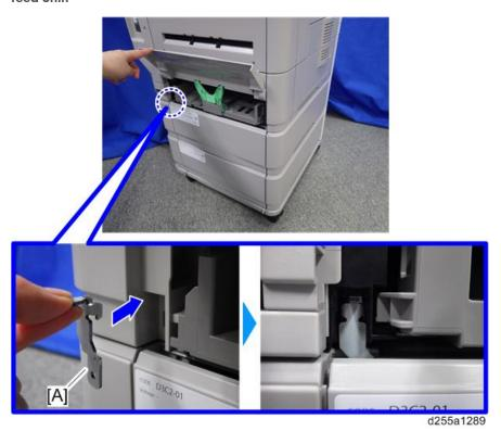
6. Open the rear cover [A] of the paper feed unit, and then secure the joint bracket installed in the previous step with the screw (M3×6).
