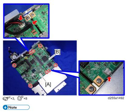
• Be careful not to damage the backside of the controller board [A] and the BiCU [B].
