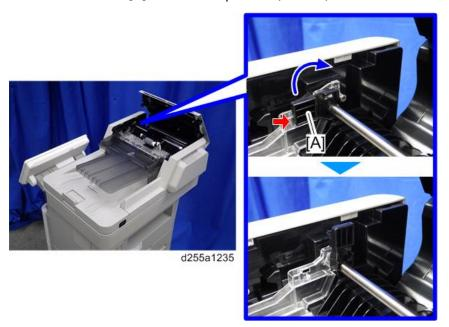
3. Remove the ARDF paper feed roller and ARDF pickup roller [A].
