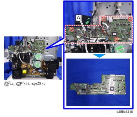
4. Remove the NVRAM [A] from the old IOB and attach it to the new IOB.
