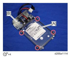
30. Disconnect the two cables [A] from the HDD [B].
