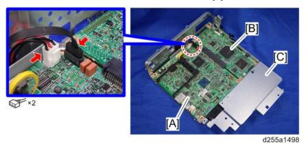
When reattaching the controller box [A], make sure to secure the harness and flat cable to the harness guides, as shown below.
