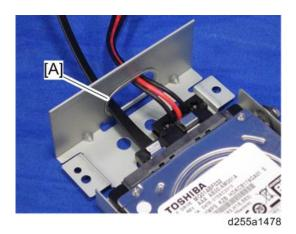
34. Install the HDD with the bracket [A] on the controller box [B]. (hook×2)
