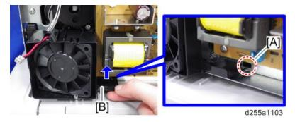
4. Remove the PSU fan with the bracket [A]. (hook×2)
