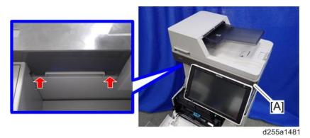
11. Insert a flathead screwdriver at [A] to release the hook, and then remove the scanner front cover [B].
