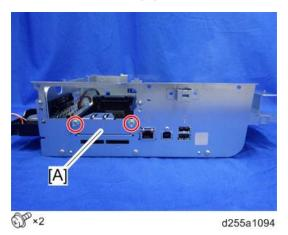
6. Remove the controller box cover [A].
