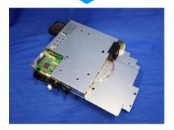
22. Disconnect the connector on the controller box [A].
