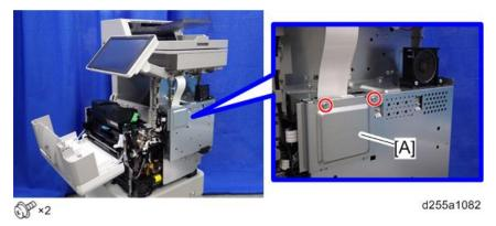
3. Disconnect the USB connector [A] of the operation panel.
