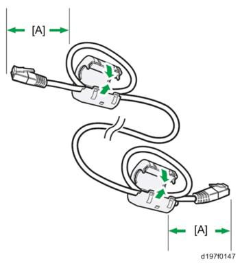
6. Only when installing this option in NA, fix each ferrite core with the cable tie [A].
