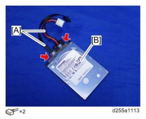
33. Install the enhanced security HDD [A] on the HDD bracket [B].
