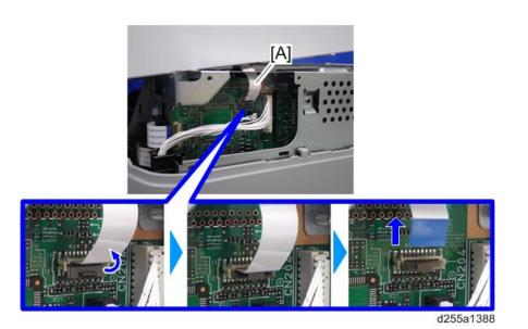
8. Remove the plastic sheet [A] from the main frame (hook×2), and then remove the upper cover [A].
