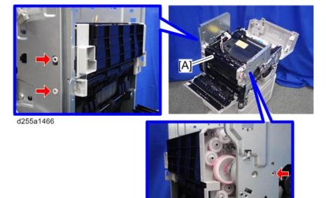
$\bullet \quad \text{When removing the paper exit unit [A], disconnect the connector [B] from the paper exit unit.}\\$
