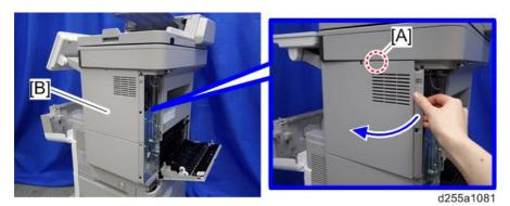
4. Remove the right upper cover [A] by inserting a flathead screwdriver into [B].
