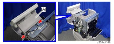
6. Insert a flathead screwdriver into [A] to release the hook, and then remove the operation panel arm upper cover [B].
