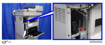
20. Connect the flat cable [A] to CN603 of the removed FCU board [B].
