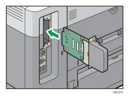
Check that the interface board is firmly connected to the controller board.
