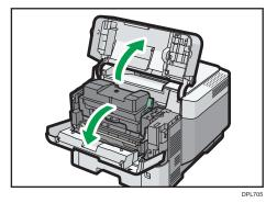
2. Hold the print cartridge with one hand as you release the print cartridge lever with another hand.
