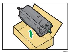
6. Shake the new print cartridge at least 10 times to the left and right so that the toner inside it spreads uniformly.
