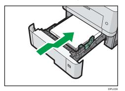
7. Lift the front side of the tray, and then slide it into the printer carefully until it stops.
