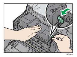
3. Squeeze the clip on the print cartridge and lift it.
