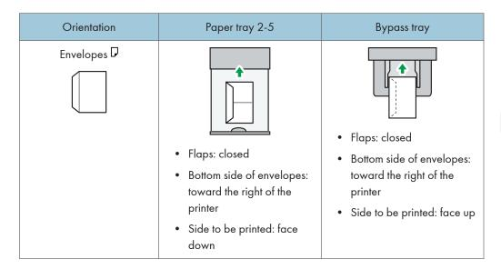
When loading envelopes, use both the control panel and the printer driver to select "Envelope" for the paper type and specify the thickness of the envelopes. For details, see page 66 "Printing on Envelopes with Windows (PCL 6/PostScript 3)", page 66 "Printing on Envelopes with Windows (PCL 5e)", and page 67 "Printing on Envelopes with OS X".
