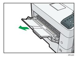
2. Load paper face up until it stops, and then adjust both sides of the paper guide to match the paper width.
