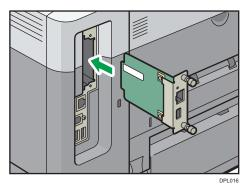
Check that the interface board is firmly connected to the controller board.
