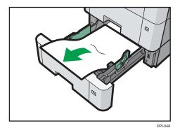
3. Hold the tray with both hands, slide it along the rails of the paper feed unit, and then push it straight in.
