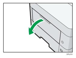
Pull the extender out when loading A4D,  $8^1/_2 \times 11D$  or larger paper.
