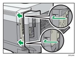
7. Hook the tab on the interface cover, which is located on the side of the rear cover.
