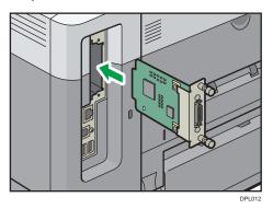
Check that the IEEE 1284 interface board is firmly connected to the controller board.
