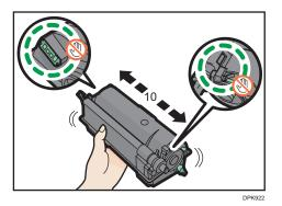
7. Insert the new print cartridge into the printer.
