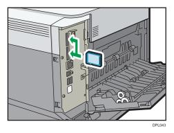
If you insert only one SD card, use the upper slot. If you insert two SD cards simultaneously, use both slots. If you insert the optional VM card, use only the lower slot.
