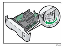
3. Squeeze the clip on the side paper guide and slide it to match the paper size.
