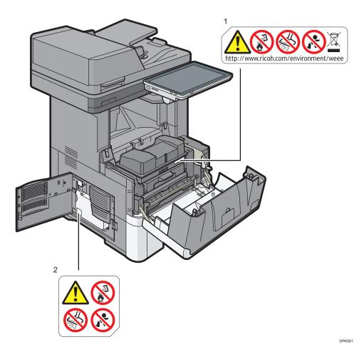
Do not incinerate toner bottles. Doing so risks burns as toner will ignite on contact with naked flame.
