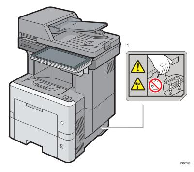
There are protruding parts on the lower side of this machine, which is near this label. Do not touch the lower part of this machine or areas near this label.
