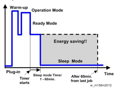
The area shaded grey in this diagram represents the amount of energy that is saved when the timers are at the default settings. If the timers are changed, then the energy saved will be different. For example, if the timers are all set to 60 min., the grey area will disappear, and no energy is saved before 60 min. expires.
