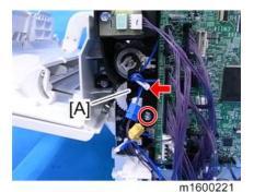
3. By-pass Feed Clutch [A] (⟨♡ x 1, 🟴 x 1)
