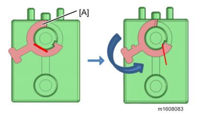
8. Slightly flex the side plates outward and pull the LED unit [A] out of the machine.
