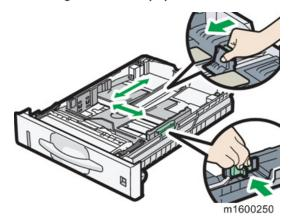
4. Load the paper, insert the tray while keeping its front slightly raised, and then push it in all the way in.
