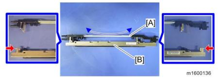
10. Remove the two spring holders [B] from the LED head [A].
