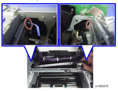
9. Bend the stay [A] to release the left and right tabs, and then separate the stay from the LED head [B].
