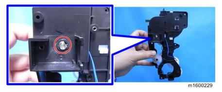
7. Toner Supply Clutch [A] with shaft (Gear x 1)
