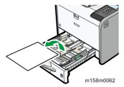
6. Pull out the paper tray, and then remove the adhesive tape [A] on its side.
