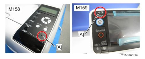
The ECO Night Sensor [A] (ambient light sensor) enables the printer to automatically turn off and on the main power when changes in the ambient light level are detected.
