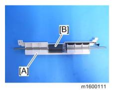
6. Separate the bypass feed roller [A] from the shaft (Hook x1).
