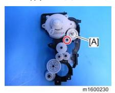
8. All things attached to the toner supply clutch [A] (Gear x 1, Shaft x 1).
