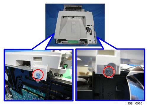
5. Remove the screws at the rear side (Fx 2).
