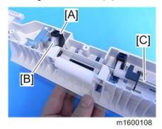
3. Push the friction pad [A] down to detach it (Spring  $\times$  1).
