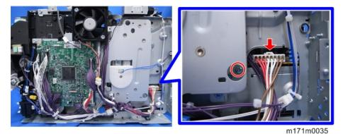
7. Two screws on the rear side of the PSU (🞯 x 2)
