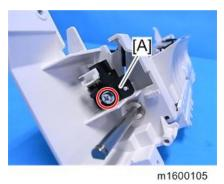
3. Detach the By-pass Paper End Sensor [A] from the bracket (Hook).
