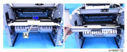
5. Detach the by-pass feed roller with the shaft [B] from the guide [A].
