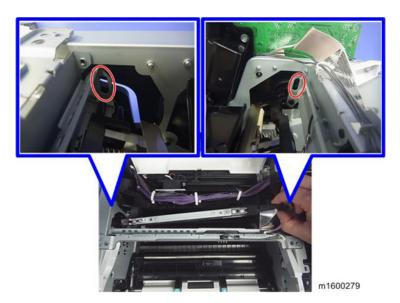
8. Bend the stay [A] to release the left and right tabs, and then separate the stay from the LED head [B].
