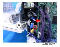
3. By-pass Feed Clutch [A] (🕅 x 1, 🞯 x 1)
