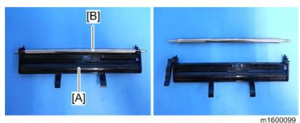
8. Detach the registration roller (driven) [B] from the guide [A].
