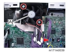
• When you reattach the PCDU cooling fan, the face of the fan with the sticker must be on the inside.
