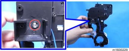
4. Toner Supply Clutch [A] with shaft (Gear x 1)
