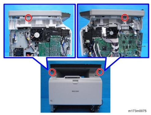
4. Lift the Scanner Unit [A] to detach from the machine.
