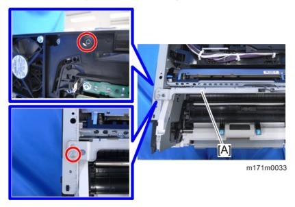
5. Rotate the LED unit [A] in the direction of the arrow until it locks.
