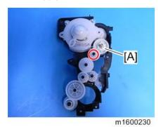
5. All things attached to the toner supply clutch [A] (Gear x 1, Shaft x 1).
