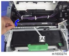
6. Remove the spacer [A], ground wire [B], and flat cable [C] from the LED unit.
