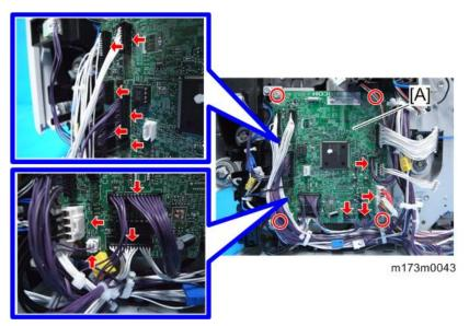
3. Remove the EEPROM [A] from the old board and install it on the new board.
