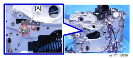
6. Insert a flathead screwdriver into the gap on the left of the registration roller guide to release the protruding part.
