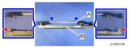
9. Remove the two spring holders [B] from the LED head [A].
