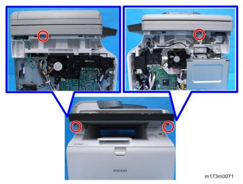
9. Lift the Scanner Unit [A] to detach from the machine.
