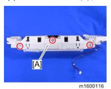
3. By-pass Bottom Plate HP Sensor [A] ( x 1, Hook)
