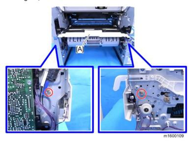
4. Slide the by-pass feed guide [A] with the by-pass feed roller to the right to detach it from the machine.
