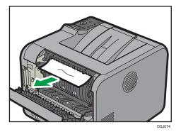
3. If you can see the jammed paper in the output tray, keep the rear cover opened and remove the paper.
