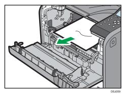
4. If you cannot see the jammed paper or remove it, lift "B" and remove the jammed paper.
