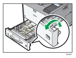
2. Pull the tray carefully until it stops, lift the front side of the tray, and then pull it out of the printer.
