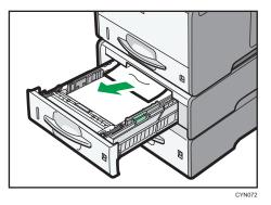
3. Hold the tray with both hands, slide it along the rails of the paper feed unit, and then push it straight in.
