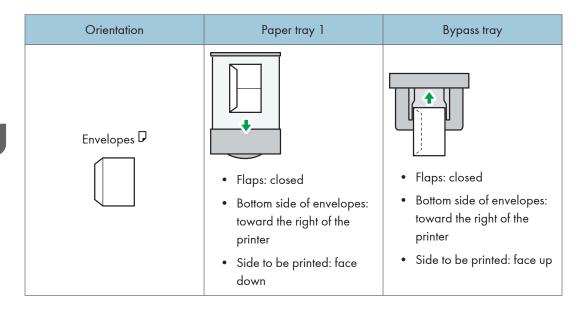
When loading envelopes, use both the control panel and the printer driver to select "Envelope" for the paper type and specify the thickness of the envelopes. For details, see page 51 "Configuring Envelope Settings Using the Control Panel".
