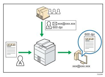
You must set up and configure a Windows server to use the distributed scan management system.
