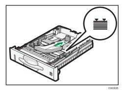
10. Pinch the clip on the side paper guide and slide it along the edge of the envelope stack.
