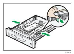
11. Pinch the end guide and slide it along the edge of the envelope stack.
