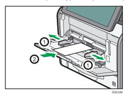
7. Adjust both sides of the paper guide to match the envelope width.
