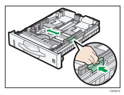
4. Pinch the end guide and slide it inward to match the standard size.
