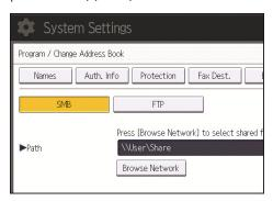
If the network does not allow automatic obtaining of IP addresses, include the destination computer's IP address in the path. For example: if the IP address of the destination computer is "192.168.0.191", and the folder name is "Share", the path will be \\192.168.0.191\Share.
