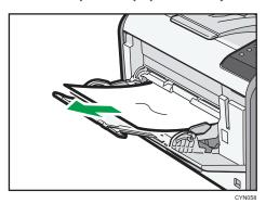
3. Open the front cover by pushing the front cover release button, and then close it to reset the misfeed condition.
