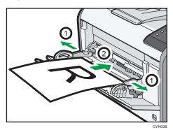
3. Adjust both sides of the paper guide to match the paper width.
