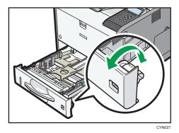
2. Pull the tray carefully until it stops, lift the front side of the tray, and then pull it out of the printer.
