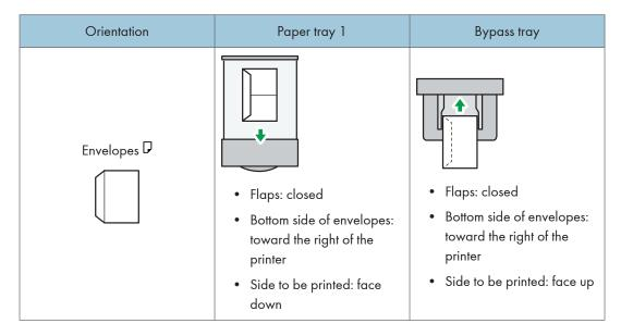
When loading envelopes, use both the control panel and the printer driver to select "Envelope" for the paper type and specify the thickness of the envelopes. For details, see page 62 "Configuring Envelope Settings Using the Control Panel".
