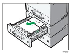
3. Hold the tray with both hands, slide it along the rails of the paper feed unit, and then push it straight in.
