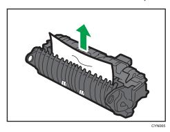
9. If the paper is not jammed in the fusing unit, remove the jammed paper from inside of the printer.
