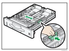
3. Pinch the clip on the side paper guide and slide it to match the paper size.
