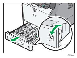
2. Pull the tray carefully until it stops, lift the front side of the tray, and then pull it out of the machine.
