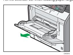
2. Slide both sides of the paper guide outward, and then load paper print side up until it stops.
