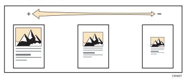
To specify a reproduction ratio, enter the ratio using the number keys or specify the ratio with [+] or [-].
