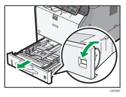
2. Pull the tray carefully until it stops, lift the front side of the tray, and then pull it out of the machine.
