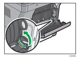
Check that paper in the paper tray is not being used, and then pull out the paper tray carefully. Adjust the paper size dial to match the size and feed direction of the paper in the paper tray.
