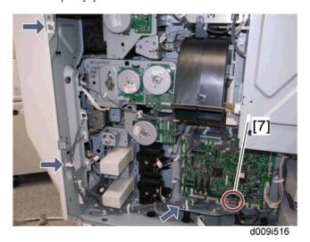
6. Connect the harness to CN211 [7] on the IOB ( $\frak{\Box} x$  3).
