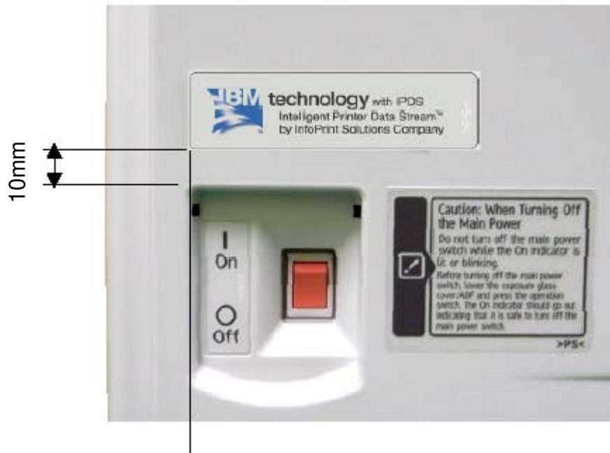
Line up the left side of the decal with the left edged of the main power switch.
