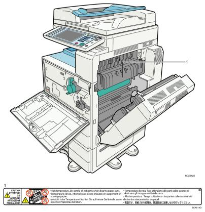
High temperature. Be careful of hot parts when clearing paper jams.
