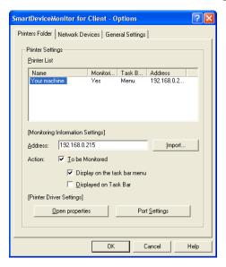
To display the machine status on the task bar, you must first select the [To be Monitored] check box, and then select the [Displayed on Task Bar] check box.
