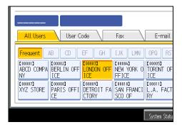
The user key is moved to the selected position, and the user key currently at the selected position is moved forward or backward.
