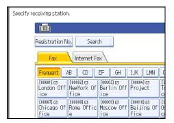
Press the key on the left of the display to switch the destination between fax number, e-mail address, Internet Fax destination, and folder destination.
