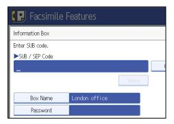
To change the SEP Code, press [Clear] or the [Clear/Stop] key, and then try again. To change the box name, press [Box Name], and then repeat the procedure from step 7.
