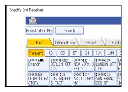
Press the key on the left of the display to switch the destination between fax number, e-mail address, Internet Fax destination, and folder destination.
