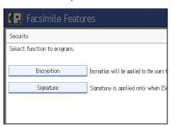
To specify encryption for documents for Forwarding, press [Encryption]. To use the encryption function, the address must be stored in the Address Book and have the encryption option enabled. For details about Encryption, consult your administrator.
