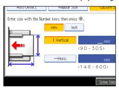
Specify a vertical size from 90 mm (3.6") to 305 mm (12.0"). You cannot enter a size smaller than 90 mm or larger than 305 mm.
