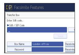
To change the SUB Code, press [Clear] or the [Clear/Stop] key, and then try again. To change Box name, press [Box Name], and then repeat from step 7.
