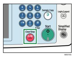
The machine stops scanning.
