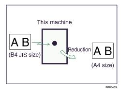
If A4 paper but not B4 paper is loaded and a B4 $\square$  document is received, the machine automatically reduces the document size so that it can be printed onto a single A4 sheet.
