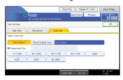
$8^{1}/_{2} \times 11$  indicates LT.  $8^{1}/_{2} \times 14$  indicates LG.  $11 \times 17$  indicates DLT.
