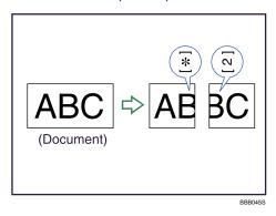
For example, this function splits the document if the document length is 20 mm (0.79 inch) or longer than the paper used. The document is reduced if it is less than 20 mm (0.79 inch). When a document is split, an asterisk ( $\bigstar$ ) is inserted at the split position and about 10 mm (0.39 inch) of the split area is duplicated on the top of the second sheet.
