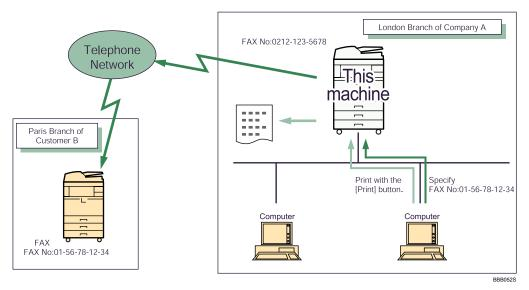
Errors occurring when the machine is used as a LAN-Fax will not be displayed on the computer. Check for errors by using a Web Image Monitor. See Web Image Monitor help.
