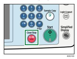
Pressing the [Clear/Stop] key deletes by single digits the fax number or IP-Fax address. The Internet Fax destination or e-mail destination can be entirely deleted at once by pressing the [Clear/Stop] key.
