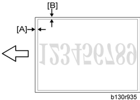
4. Measure the distance between the leading edge of the image area and the leading edge of the paper [A].
