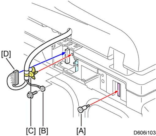
2. Remove the stud screw [A].
