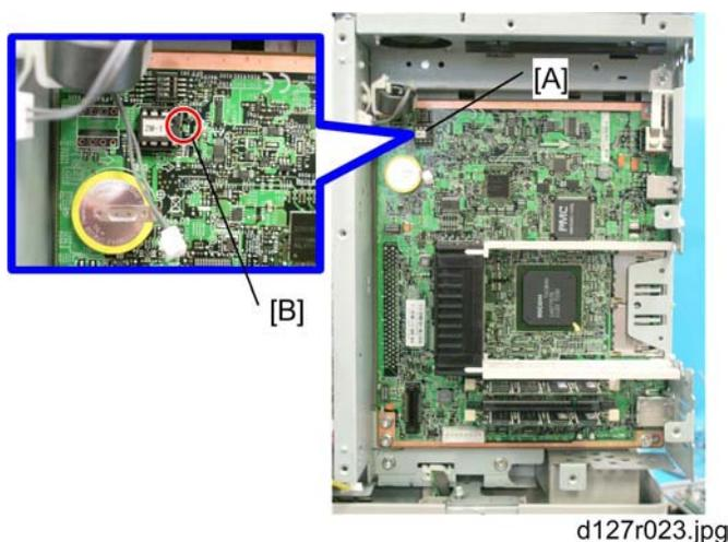
2. Install a New NVRAM on the controller. Then reassemble the machine.
