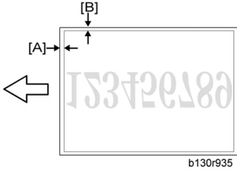
3. Measure the distance between the leading edge of the image area and the leading edge of the paper [A].
