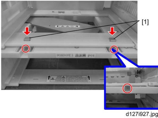
1. Attach the joint bracket (Front) [1] as shown. (🔧 x 2)
