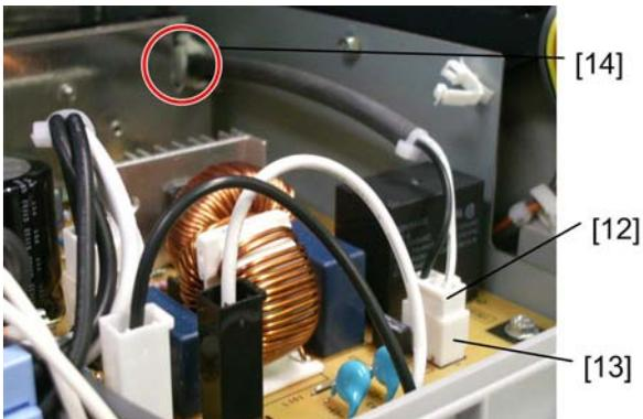
12. Attach the heater harness (Long) [12] to the connector [13] on the board.
