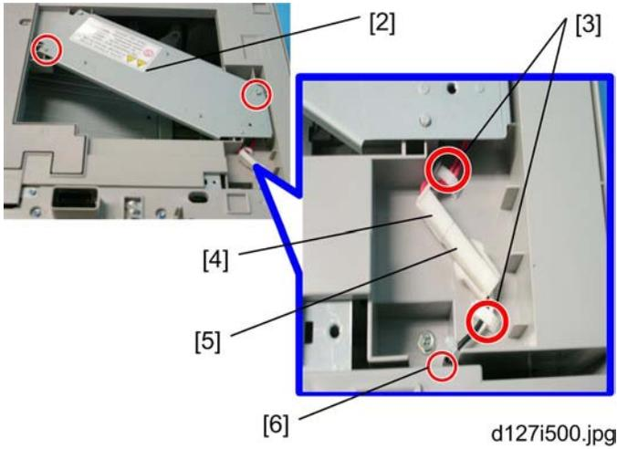
3. Attach the heater [2] to the lower paper tray unit (
