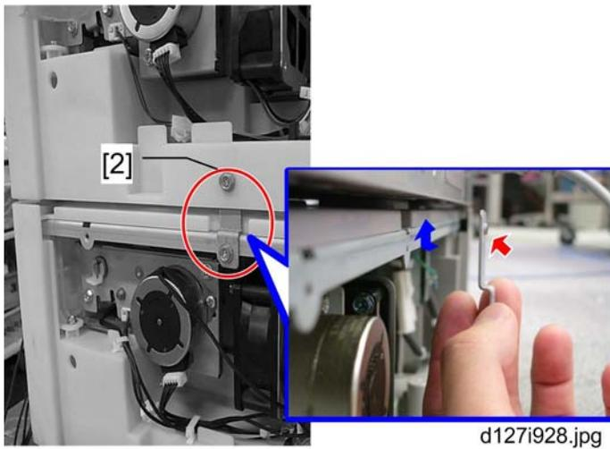
2. Attach the joint bracket (Rear) [2] as shown. (🔧 x 2)
