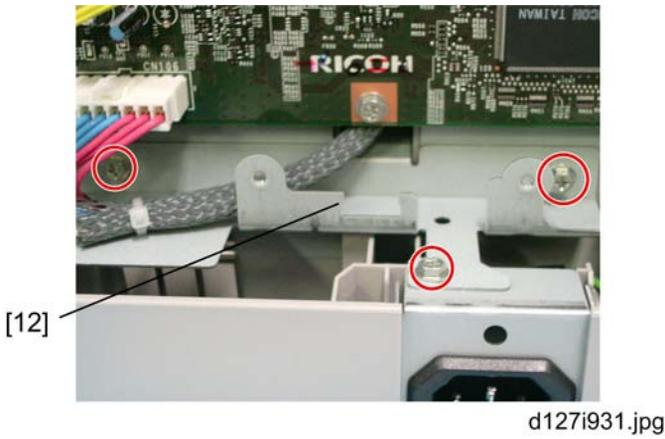
12. Remove the support bracket [12] (🛠️ x 3).
