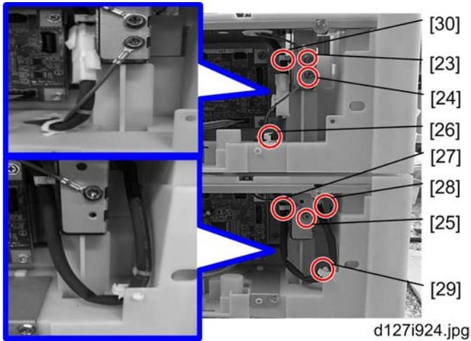
28. Attach the grounding wire (Long) [23] (
