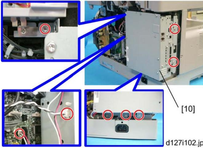
10. Remove the controller box [10] (🔩 x 2, 🛠️ x 6).
