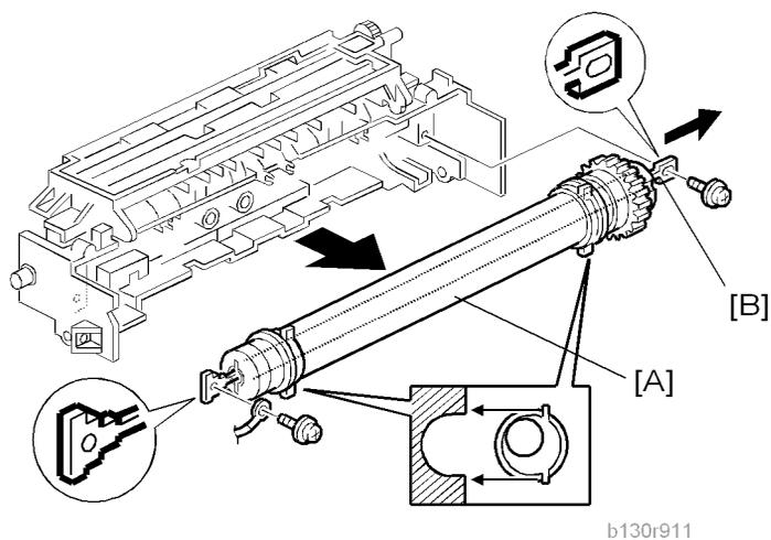
1. Hot roller stripper pawls and spacers (p.87 "Hot Roller Stripper Pawls")
