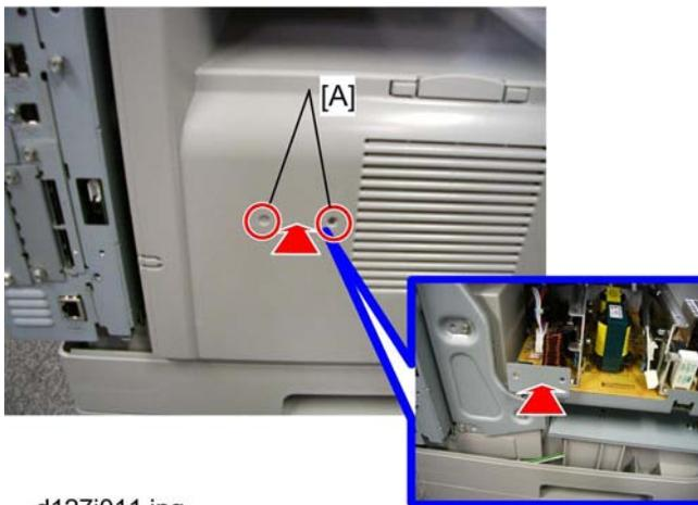
1. Make two holes [A] through which the screws fasten the handset bracket to the main machine. (Just penetrate with a screw driver)
