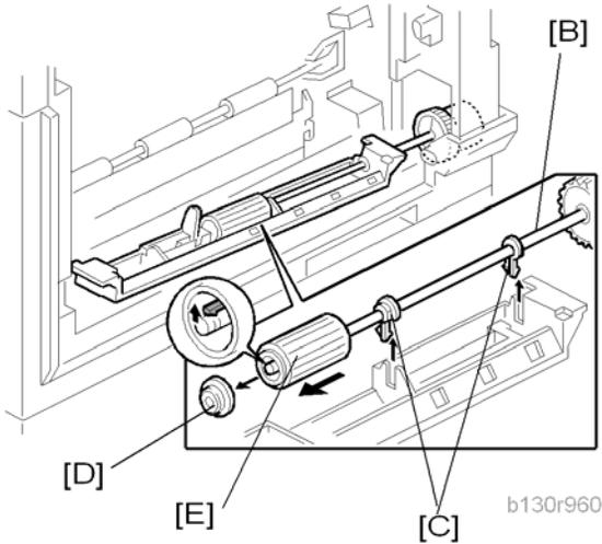
3. Feed roller shaft [B] (2 snap pawls [C], 1 spacer [D])
