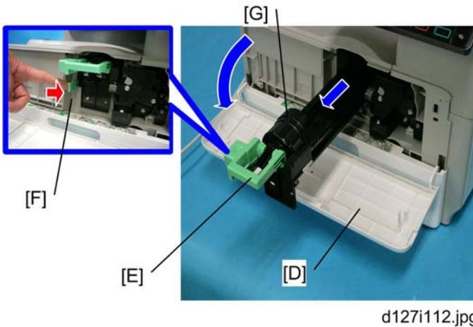
5. Lift lever [E], press in on latch [F] and pull the bottle holder [G] out. (You do not need to pull it completely out of the machine.)
