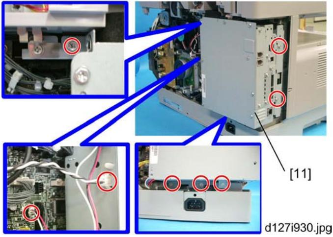
11. Remove the controller box [11] (🔧 x 2, 🛠️ x 6).
