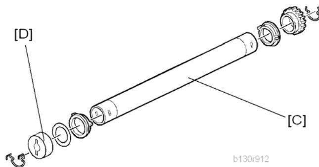
4. Hot roller [C] (2 C-rings, 1 spacer, 1 gear, 2 bushings, 1 cover [D])
