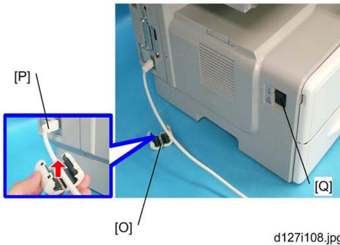
21. Attach the ferrite core [O] to the end of the network cable [P] when connecting the cable.
