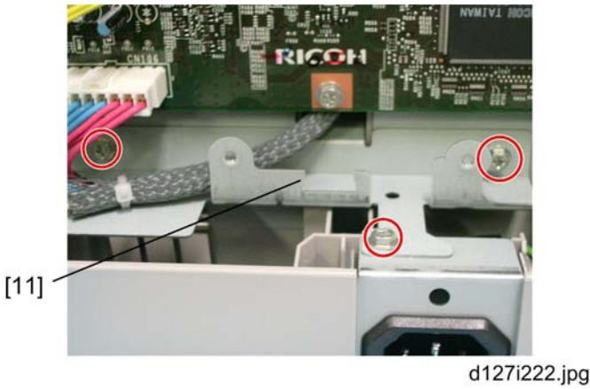
11. Remove the support bracket [11] (🛠️ x 3).
