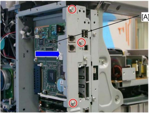
5. Remove three of the screws and pull the bracket as the arrow shows to detach the board [A].
