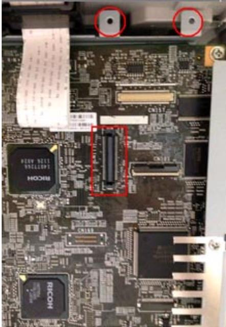
7. Attach the copy data security unit board with bracket to CN111.
