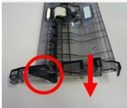
4. Replace the separation cushion (with P/N D6063119) **OR**, cut off the portion of the Mylar that is sticking out.
