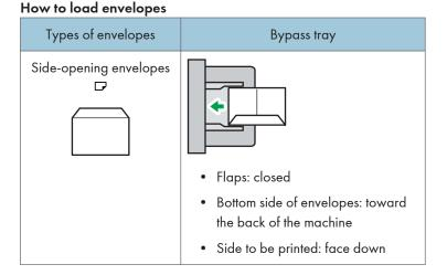
When loading envelopes, select "Thick Paper" as the paper thickness and "Plain Paper" as the paper type using both the User Tools and printer driver. For details, see "Printing on Envelopes", Print<sup>®</sup>.
