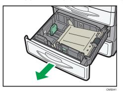
2. While pressing down the release lever of the side fence, slide the side fence outward.
