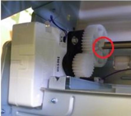
4. Shift the drive gear to the side (in the direction of the red arrow) while holding the up-and-down frame.
