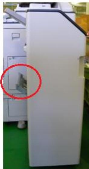
5. Remove the base frames (4 screws).
