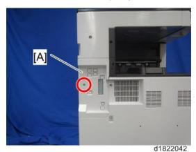
2. Insert the PS3 SD card in SD card slot 2 [A].
