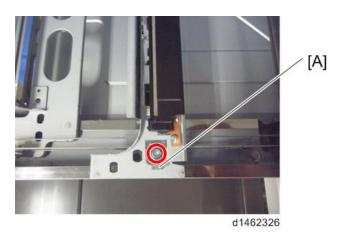
10. Remove the wire fixing bracket [A] and the spring [B] (  $\hspace{-0.5cm}\widehat{\hspace{-0.5cm}/}\hspace{-0.5cm} x1$  ).
