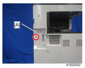
7. Install the guide rail [A] in the front frame of the main machine ( $\mathfrak{F}$  bind screw x 3; M3 x 6).
