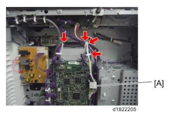
9. Pass the harness from the optional counter device through the cut off part of the right rear cover. Coil the rest of the harness and put it on the space above the BCU bracket.
