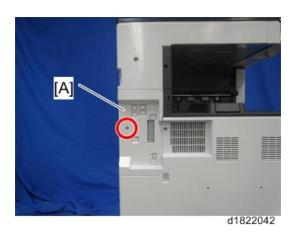
3. Insert the SD card into SD Card Slot 2 [A]. Make sure the label on the SD card faces the front side of the machine.
