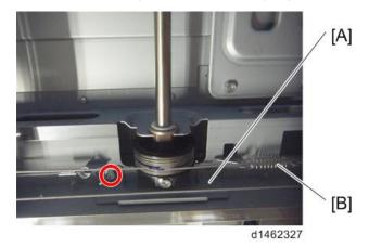
11. Remove the wire pulley [A] ( $\mathscr{F}x1$ , ( )x1).
