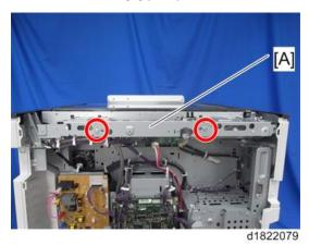
3. Remove the SIO [A] ( \$\begin{align\*} x4, \quad x7 \end{align\*}.
