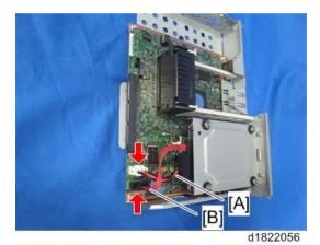
5. Reinstall the controller board with the HDD.
