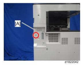
2. Remove the knockout [A] (USB) from the controller cover.
