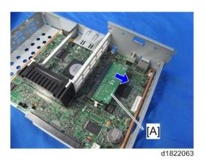
5. Align the position of the cutout and insert the memory unit into the memory board slot at a slant.
