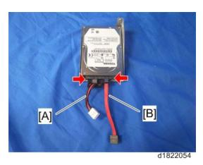
3. Hang the HDD [A] on the hook [B] of the controller box and secure it ( $\mathscr{F}x3$ ).
