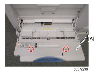
3. Replace the by-pass paper length sensor [A] ( 1).
