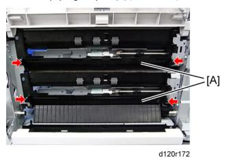
4. Replace the separation roller [A] (🖾x1).
