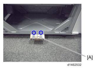
16. Attach the connecting bracket that comes with the finisher adapter [A] to the finisher (Fx1: M4×25: supplied with the finisher adapter).
