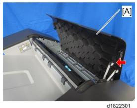
8. Remove the auxiliary cover [A] from the top cover (hooks x 2,  $\mathscr{F}$ x2).
