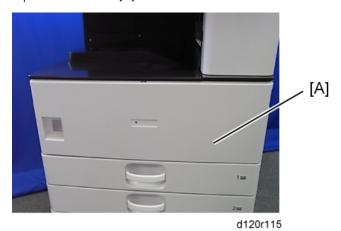
2. Remove the two pins [A], and then remove the front cover.
