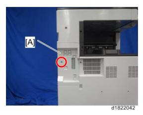
2. Remove the cover [A] of the board slot (  $\slash\hspace{-0.6em}\widehat{\hspace{-0.5em}/}\hspace{-0.4em} x1$  ).
