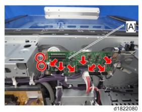
4. Remove the bracket [A] ( \*x4, \subsetext{\$\subset}x3).
