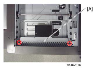
3. Remove the lens block [A] ( \$\begin{aligned} \pi x5, & \pi x2 \end{aligned}.
