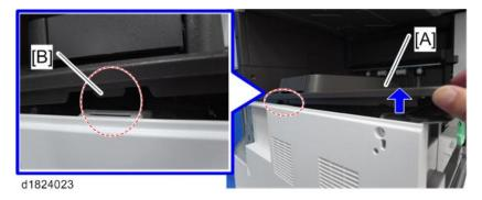
5. Remove the left cover [A] upward.
