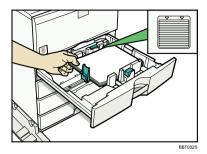
While pressing the release lever, push in the side and end fences until they are flush against the paper's edges.
