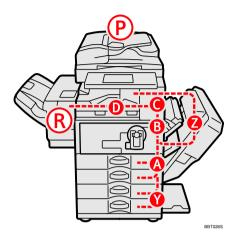
1. Press the key of the section from where you want to remove the jammed paper.
