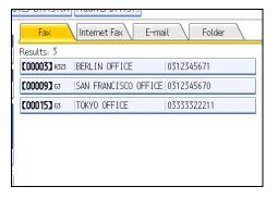
If the destination you require does not appear, use [▲] or [▼] to scroll through the list. Press [Details] to display the details of a selected destination.
