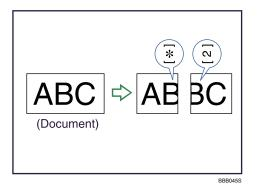
For example, this function splits the document if the document length is 20 mm (0.79 inch) or longer than the paper used. The document is reduced if it is less than 20 mm (0.79 inch). When a document is split, an asterisk (★) is inserted at the split position and about 10 mm (0.39 inch) of the split area is duplicated on the top of the second sheet.
