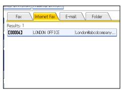
If the destination you require does not appear, use [▲] or [▼] to scroll through the list. Press [Details] to display the details of a selected destination.
