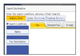
3. Press the transmission type tab to switch the transmission type to fax/IP-Fax, Internet Fax, e-mail, or folder.
