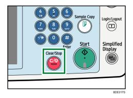
Pressing the [Clear/Stop] key deletes by single digits the fax number or IP-Fax address. The Internet Fax destination or e-mail destination can be entirely deleted at once by pressing the [Clear/Stop] key.
