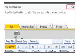
Press the transmission type tab to switch the transmission type between fax/IP-Fax, Internet Fax, email, or folder.
