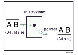
If A4<sup>D</sup> paper is loaded and a document of B4 JIS<sup>D</sup> size is received, the machine will reduce the document to a single A4<sup>D</sup> sheet.
