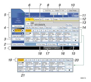
1. Displays the date, time, and machine status. Displays the name, facsimile number of the destination, and the size of the original when transmitting.
