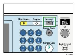
The interrupt key indicator lights. The machine stops scanning.
