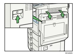
2. Push down the green lever of the fusing unit on the left.
