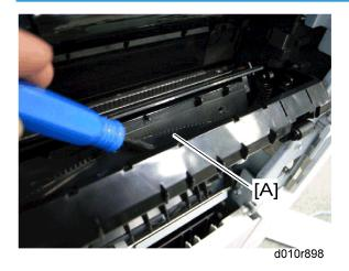
1. Insert the new discharge plate [A] into the image transfer unit as shown.
