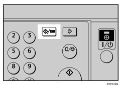
**2** Select [Fax Features] using [▲] or [▼], and then press the [OK] key.
