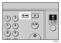
**2** Select [System Settings] using [ $\blacktriangle$ ] or [ $\checkmark$ ], and then press the [OK] key.
