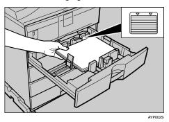
**1** While pressing the release lever, push in the side and end fences until they are flush against the paper's edges.
