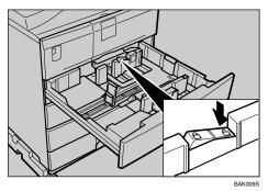
**6** While pressing the release lever, slide the side fences outward.
