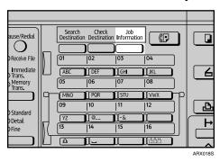
2 Select [Print TX Standby File List] using [▲] or [▼], and then press the [OK] key.
