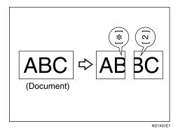
For example, this function splits the document if the document length is 20 mm (0.79") or longer than the paper used. The document is reduced if it is less than 20 mm (0.79"). When a document is split, an asterisk ( $\bigstar$ ) is inserted at the split position and about 10 mm (0.39") of the split area is duplicated on the top of the second sheet.
