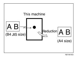
If A4 $\square$  paper is loaded and a document of B4 JIS $\square$  size is received, the machine will reduce the document to a single A4 $\square$  sheet.
