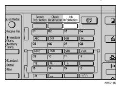
**2** Select [TX File Status] using [▲] or [▼], and then press the [OK] key.
