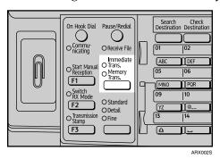
Check the indicator on the operation panel to see which mode is currently active.
