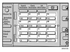
Flip the Quick Dial Flip Plate down to access Quick Dial keys 01 through 16, flip up to access keys 17 through 32.
