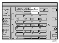
**2** Select [Check/Stop TX File] using [▲] or [▼], and then press the [OK] key.
