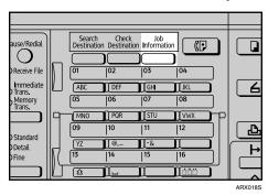
**2** Select [RX File Status] using [▲] or [▼], and then press the [OK] key.
