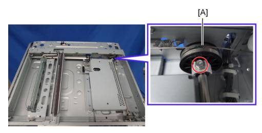
9. Remove the rear scanner drive pulley [A] (  $\slash\hspace{-0.4em}P \times 1$  ).
