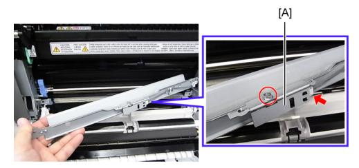
5. Remove the registration sensor bracket [A] (  $\rat{P}$  x1,  $\rat{L}$  x1).
