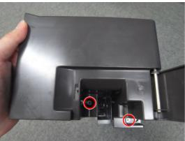
16. Open the punch cover's front door [A], and then secure the punch cover to the punch unit ( \*\* x 2: M3x6).
