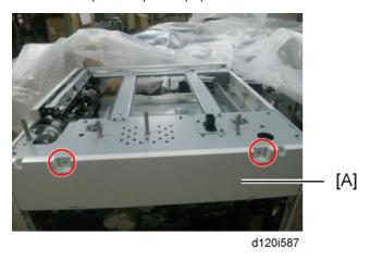
1. Remove the rear cover [A] of the optional paper feed unit (  $\mbox{\ensuremath{\not{p}}}\xspace x 2).$
