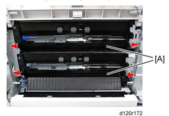
3. Remove the paper guide plate [A] (tab x 2 each).
