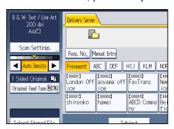
The selected destination is highlighted and also is displayed in the destination field at the top of the
