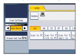
Note that only [Erase Border] can be specified directly from this machine. Use the client computer to configure the other scan settings. For details, see "Changing a Scan Profile".
