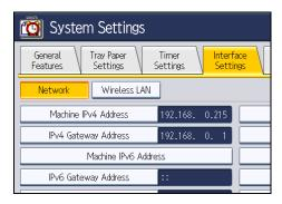
3. Press [Machine IPv4 Address] to specify the machine's IPv4 address.
