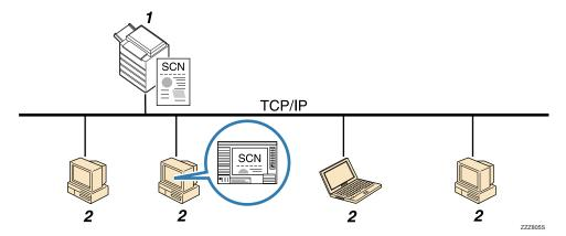
Scans an original after receiving a scan instruction from a client computer, and then sends the scan file over the network to the client computer.
