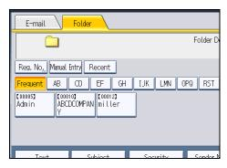
2. Enter the five-digit registration number that has been assigned to a destination folder using the number keys.
