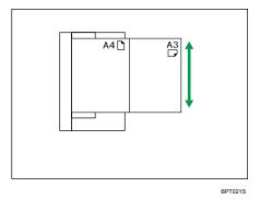
• If you do not select [Mixed Original Sizes] and place originals of different sizes in the ADF, paper jams might occur or parts of the originals might not be scanned.
